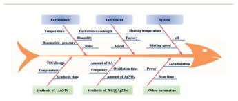
**Fig. 1** Fishbone diagram of CPPs affecting the performance of Au@AgNPs.
