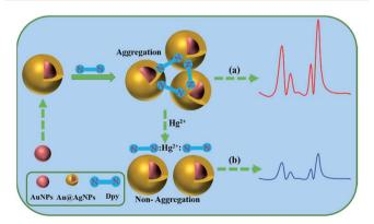
Scheme 1 Schematic illustration of the fabrication of Au@Ag-Dpy SERS probe and a sensing protocol for Hg<sup>2+</sup>. (a) Indicates the SERS signal without the addition of mercury ions; (b) indicates the SERS signal after the addition of mercury ions.
