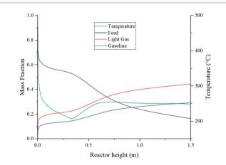
Fig. 12 Composition and temperature profiles vs. reactor height.
