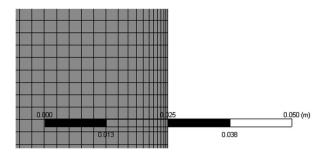
Fig. 3 Inflation method close up view
