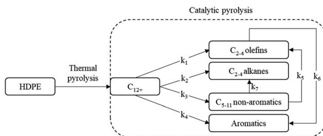
Fig. 2 Kinetic scheme for the reaction. Adapted from Artetxe *et al.*<sup>8</sup>
