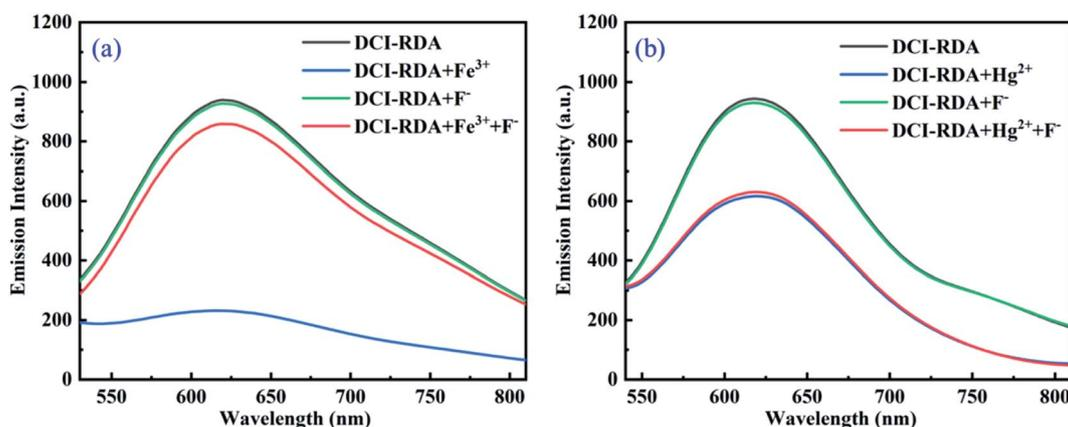
Fig. 4 Fluorescence emission spectra of the DCI-RDA solution with different additives (a) 280 μM Fe<sup>3+</sup>, 340 μM F<sup>-</sup>; (b) 22 μM Hg<sup>2+</sup>, 66 μM F<sup>-</sup> in ethanol solution, respectively. EX slit: 5.0 nm EM slit: 10.0 nm,  $T = 25\text{ }^{\circ}\text{C}$ .
