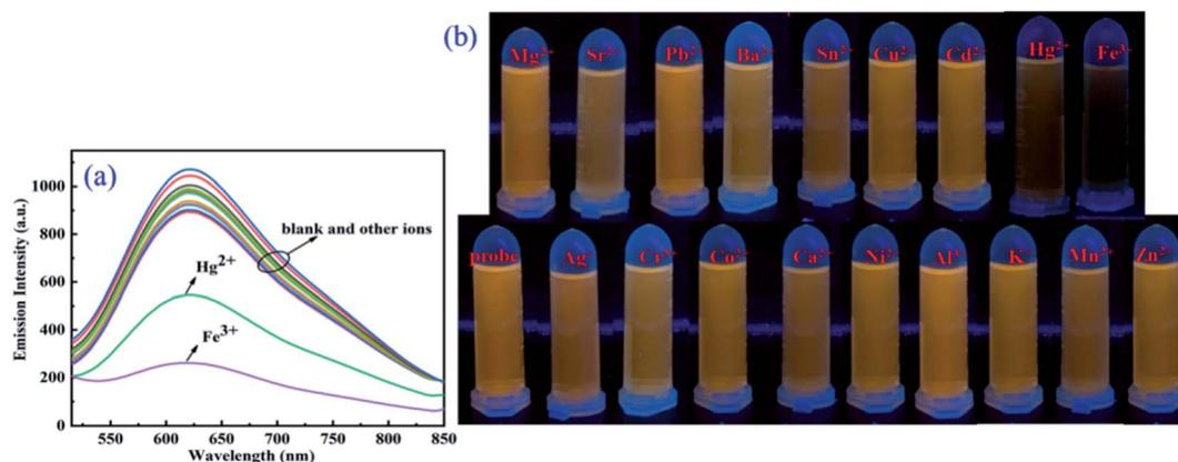
Fig. 2 (a) Fluorescence spectra of probe DCI-RDA (20  $\mu\text{M}$ ) with various metal ions (280  $\mu\text{M}$ ) in ethanol solution; (b) color changes of the DCI-RDA solution (20  $\mu\text{M}$ ) with various metal ions (280  $\mu\text{M}$ ) added under a UV-vis lamp (365 nm). EX slit: 5.0 nm, EM slit: 10.0 nm,  $T = 25^\circ\text{C}$ .
