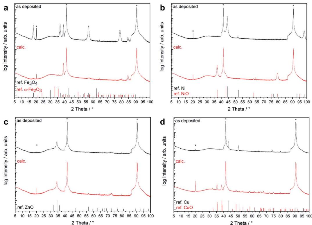
Fig. 4  $\theta$ - $2\theta$  X-ray diffraction pattern of thin films grown on  $\text{Al}_2\text{O}_3(0001)$  at  $500^\circ\text{C}$  using the different precursors 1–4 before (as deposited) and after calcination (calc.). The vertical lines mark the reference values for the identified crystalline phases.
