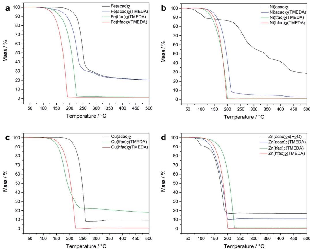
Fig. 2 Dynamic TGA curves for  $[M(\text{acac})_2]_n$ ,  $M(\text{acac})_2(\text{TMEDA})$ ,  $M(\text{tfac})_2(\text{TMEDA})$  and  $M(\text{hfac})_2(\text{TMEDA})$  ( $M = \text{Fe}$  (a),  $\text{Ni}$  (b),  $\text{Cu}$  (c) and  $\text{Zn}$  (d)).
