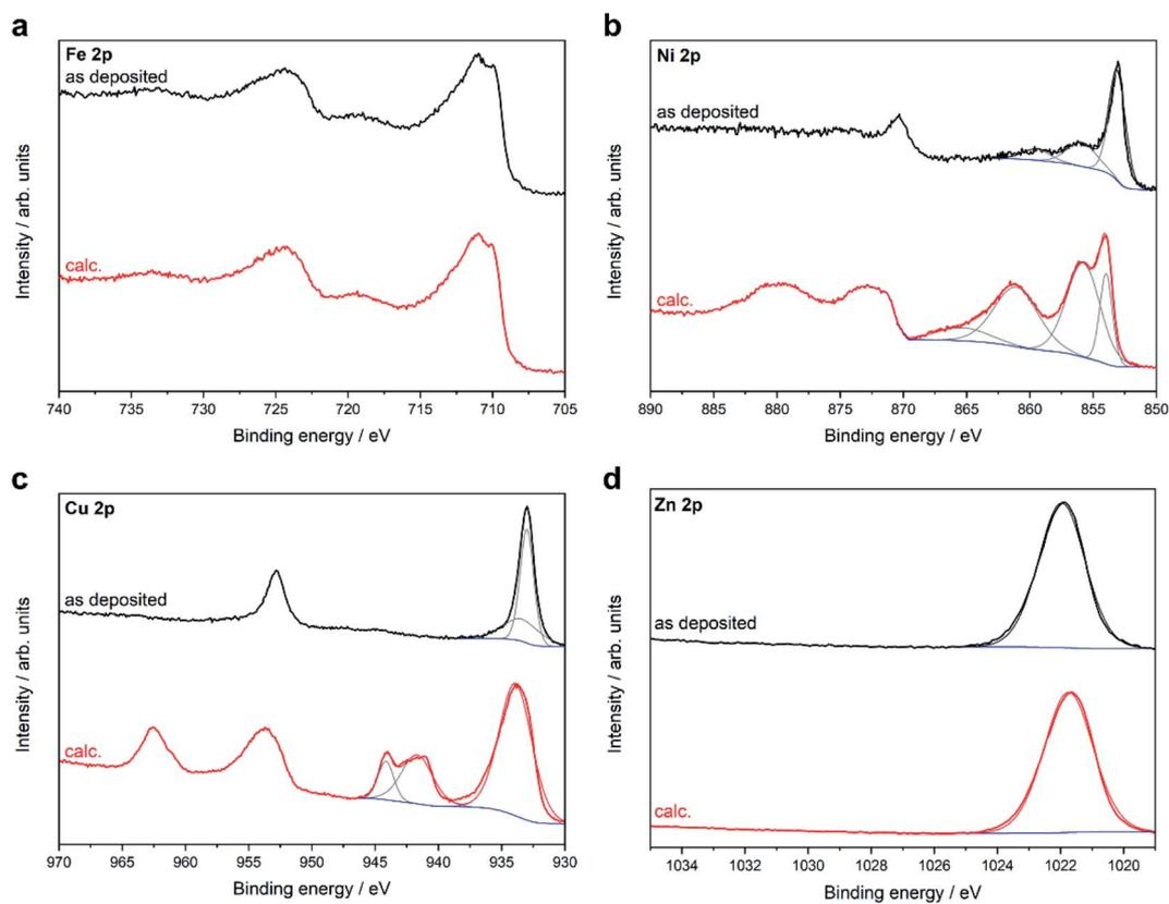
Fig. 6 XPS core level metal 2p spectra of thin films grown on  $\text{Al}_2\text{O}_3(0001)$  at  $500\text{ }^\circ\text{C}$  using the different precursors 1–4 before (as deposited) and after calcination (calc.).
