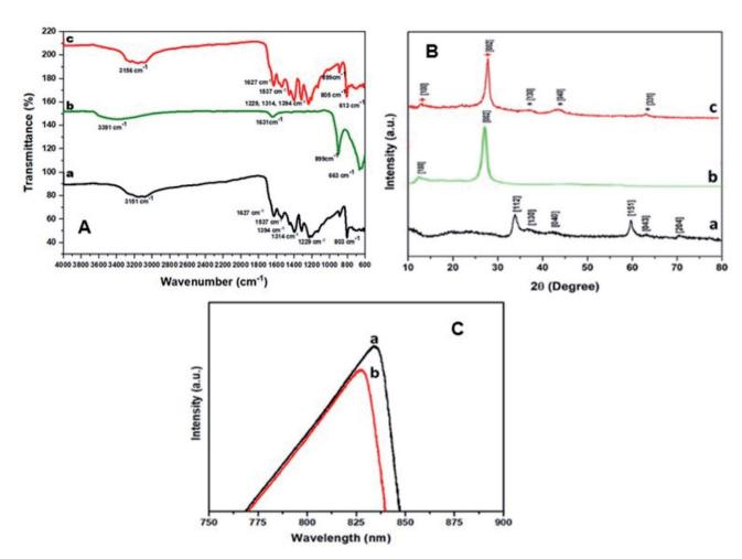
Fig. 2 (A) FTIR spectra of (a)  $g-C_3N_4$ , (b)  $NiCr_2O_4$ , and (c)  $NiCr_2O_4/g-C_3N_4$  composite. (B) XRD patterns of (a)  $g-C_3N_4$ , (b)  $NiCr_2O_4$ , and (c)  $NiCr_2O_4/g-C_3N_4$  composite. (C) PL spectra of (a)  $g-C_3N_4$  and (b)  $NiCr_2O_4/g-C_3N_4$  composite.
