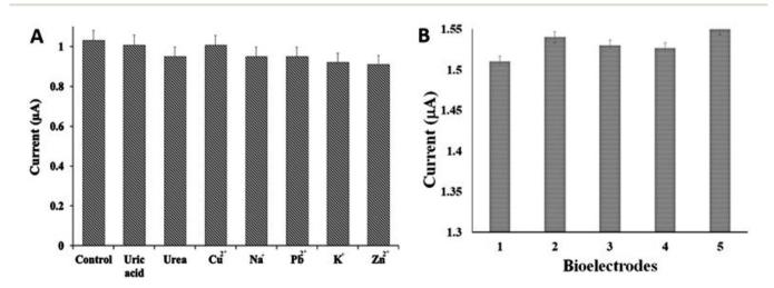
Fig. 9 (A) CV current responses in pH 7.4 PBS containing 2 mM ATCl without and with the interfering substances. (B) CV current responses of five bioelectrodes in pH 7.4 PBS containing 2 mM ATCl to test the reproducibility of the results.
