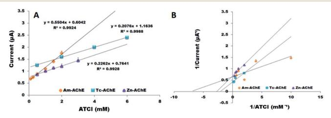
Fig. 7 (A) Calibration curves of ATCl in pH 7.4 PBS for Am-AChE/Ni/GCN/PGE (a), Tc-AChE/Ni/GCN/PGE (b), and Zn-AChE/Ni/GCN/PGE (c); (B) the Lineweaver–Burk plot of 1/current vs. 1/ATCl for Am-AChE/Ni/GCN/PGE (a), Tc-AChE/Ni/GCN/PGE (b), and Zn-AChE/Ni/GCN/PGE (c).
