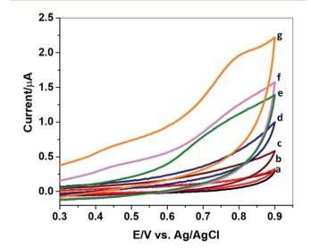
Fig. 5 Cyclic voltammograms of bare PGE in pH 7.4 PBS (a), bare PGE in pH 7.4 PBS containing ATCl (b), Ni/GCN/PGE in pH 7.4 PBS (c), Ni/GCN/PGE in pH 7.4 PBS with ATCl (d), Zn-AChE/Ni/GCN/PGE (e), Tc-AChE/Ni/GCN/PGE (f), and Am-AChE/Ni/GCN/PGE (g) in pH 7.4 PBS containing ATCl.
