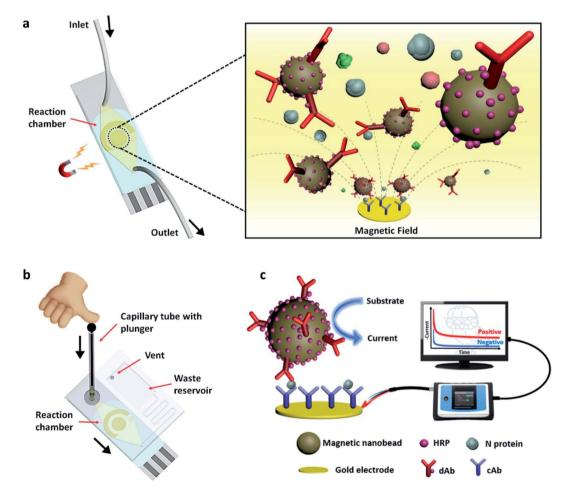
Fig. 9 (a) Simple illustration of the surface of the nano-biosensor, (b) test procedure, and (c) the complete setup of the device. In the figure, HRP, dAb, and N protein stand for horseradish peroxidase, detection antibody, and nucleocapsid proteins, respectively. Reprinted (adapted) with permission from (ref. 51) copyright 2021, ACS.
