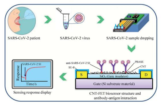
Fig. 6 CNT-FET-based nano-biosensor and SARS-CoV-2 S1 detection process. Reprinted (adapted) with permission from (ref. 40) copyright 2022, Elsevier.
