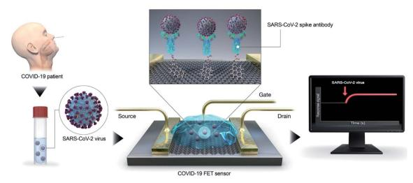
Fig. 3 Simple illustration of an immuno-biosensor manufactured by coating the graphene sheet of a FET with a clearly defined protein found in coronavirus spikes. Reproduced (adapted) from (ref. 30) copyright 2020, ACS.
