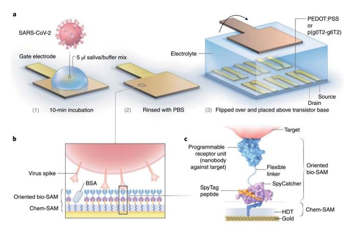
Fig. 5 (a) Functionalities of sensors, (b) different layers for operation purposes, and (c) the molecular structure of proposed nano-biosensors. Reprinted (adapted) with permission from (ref. 37) copyright 2021, Springer Nature.
