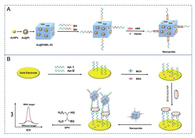
Fig. 13 Schematic depiction of the fabrication processes for the nanoprobes (A) and the electrochemical aptasensor for the capture and detection of 2019-nCov-NP (B). Reprinted (adapted) with permission from (ref. 59) copyright 2021, Elsevier.
