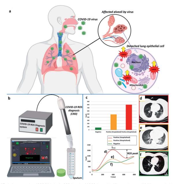
Fig. 4 (a) Typical representation of ROS, (b) device for ROS detection, (c) ROS detected in different patients, and (d), (e) contrasted with a verified sample. (f) Red, orange, and green represent 800 μA, 490 μA, and ~71 μA, respectively. Images produced by lung CT scanning (d, e, and f). Reprinted (adapted) with permission from (ref. 10) copyright 2021, Elsevier.
