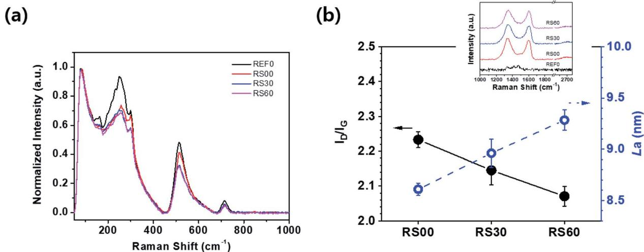
Fig. 4 Raman spectra of four dielectric films, *i.e.*, REF0, RS00, RS30, and RS60, respectively. (a) Raman spectra of the BTO peaks, and (b) the variation between  $I_D/I_G$  ratio and  $L_a$  corresponding to the sonication time. Inset is typical Raman spectra of rGO peaks.
