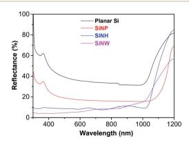
Fig. 4 Reflectance spectra of planar Si, SiNPs, SiNHs and SiNWs in the incident wavelength range from 500 to 1200 nm.
