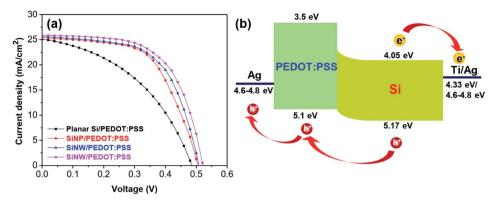
Fig. 5 (a) J-V characteristic curves of the hybrid solar cell using planar Si and Si nanostructures and (b) energy diagram of the n-Si/PEDOT:PSS hybrid solar cell.
