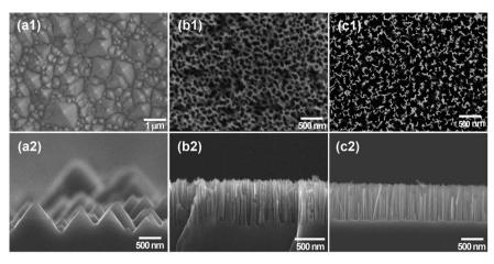
Fig. 2 SEM images of the top-viewed and cross sectional viewed (a1 and a2) SiNPs, (b1 and b2) SiNHs and (c1 and c2) SiNWs.
