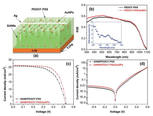
Fig. 7 (a) Structure, (b) EQE spectrum, (c) J-V characteristic curves and (d) dark J-V curves of SiNW/PEDOT:PSS/AuNPs hybrid solar cells.
