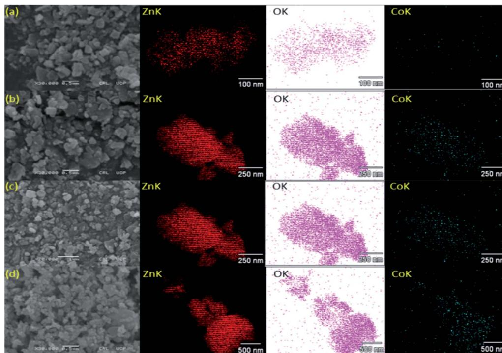
Fig. 2 SEM images of Co–ZnO,  $x = 0$  (a),  $x = 0.01$  (b),  $x = 0.05$  (c),  $x = 0.09$  (d).
