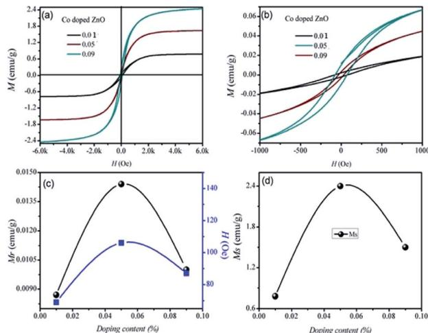
Fig. 5 (a) The  $M(H)$  loops versus Oe measured at 300 K for Co-ZnO nanoparticles (b) The inset is the  $M(H)$  loops close zero magnetic fields, (c) The  $M_r$  and  $H_c$  versus doping content, and (d) saturation magnetization versus doping content for  $\text{Zn}_{1-x}\text{Co}_x\text{O}$  with different doping concentration  $x = 0.00$ ,  $0.05$ ,  $0.09$  and  $0.09$ .
