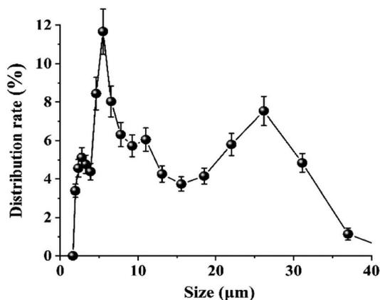
Fig. 3 Particle size distribution of the expansive soil.
