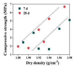
Fig. 7 Dry density – compressive strength graph.
