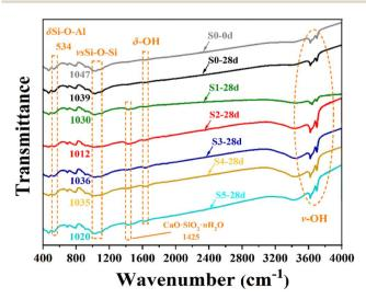
Fig. 12 FTIR characterization of samples.
