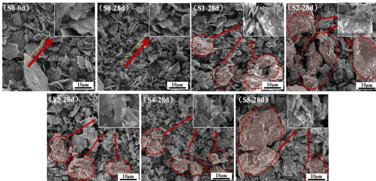
Fig. 13 SEM characterization of samples (red area surrounded by circle indicated aggregates of soil particles and arrows point to indicated morphological features of the aggregates when magnified).
