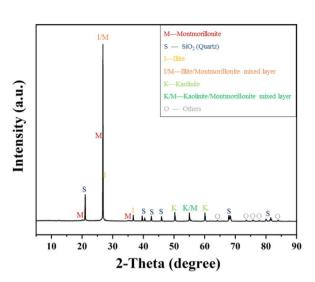
Fig. 2 XRD characterization of the expansive soil
