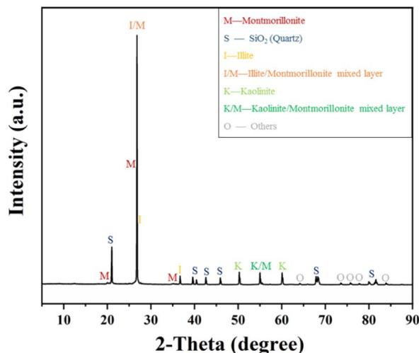
Fig. 2 XRD characterization of the expansive soil.
