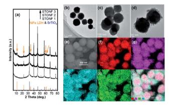
Fig. 1 (a) PXRD pattern of as-prepared catalysts (orange arrows show the peaks of NiFe LDH); (b) TEM image of as-prepared SrTiO $_3$ ; (c and d) TEM images of STONF 2; (e) SEM image of STONF 2; (f–i) EDS element mappings of selected area; (j) overlapping image of (e–i).
