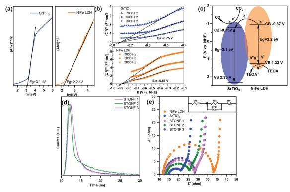
Fig. 4 (a) Tauc plots and (b) Mott-Schottky plots of SrTiO<sub>3</sub> and NiFe LDH; (c) schematic illustration of band structure alignment in STONFs composites; (d) transient PL decays and (e) Nyquist plots of as-prepared catalysts.
