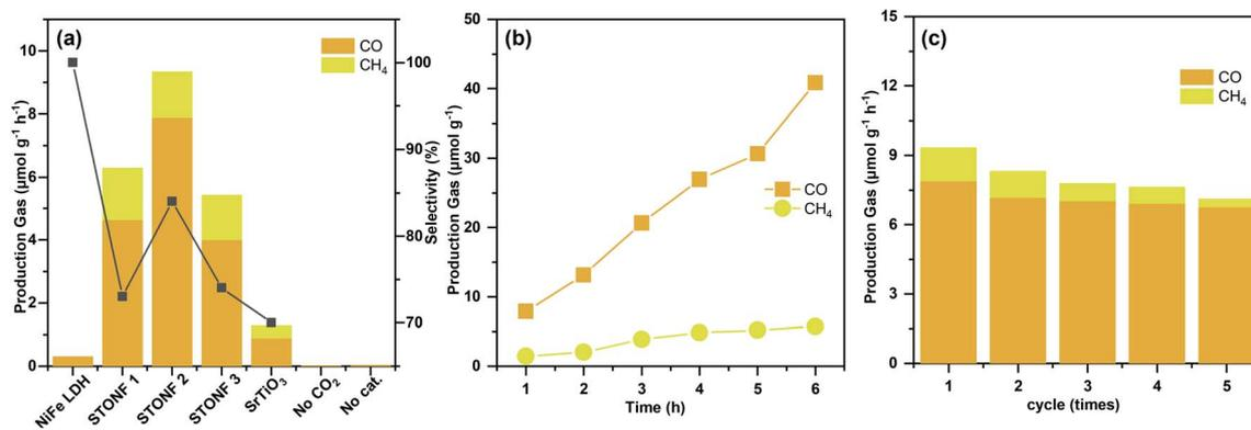
Fig. 2 (a) Production gas amount and corresponding CO selectivity of as-prepared catalysts; (b) time-dependent production gas amount of STONF 2; (c) recycling test of STONF 2 for 5 times with CO<sub>2</sub> refilled every 3 h.
