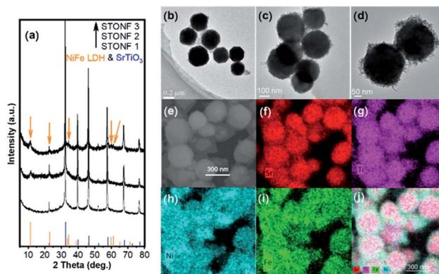
Fig. 1 (a) PXRD pattern of as-prepared catalysts (orange arrows show the peaks of NiFe LDH); (b) TEM image of as-prepared SrTiO<sub>3</sub>; (c and d) TEM images of STONF 2; (e) SEM image of STONF 2; (f-i) EDS element mappings of selected area; (j) overlapping image of (e-i).
