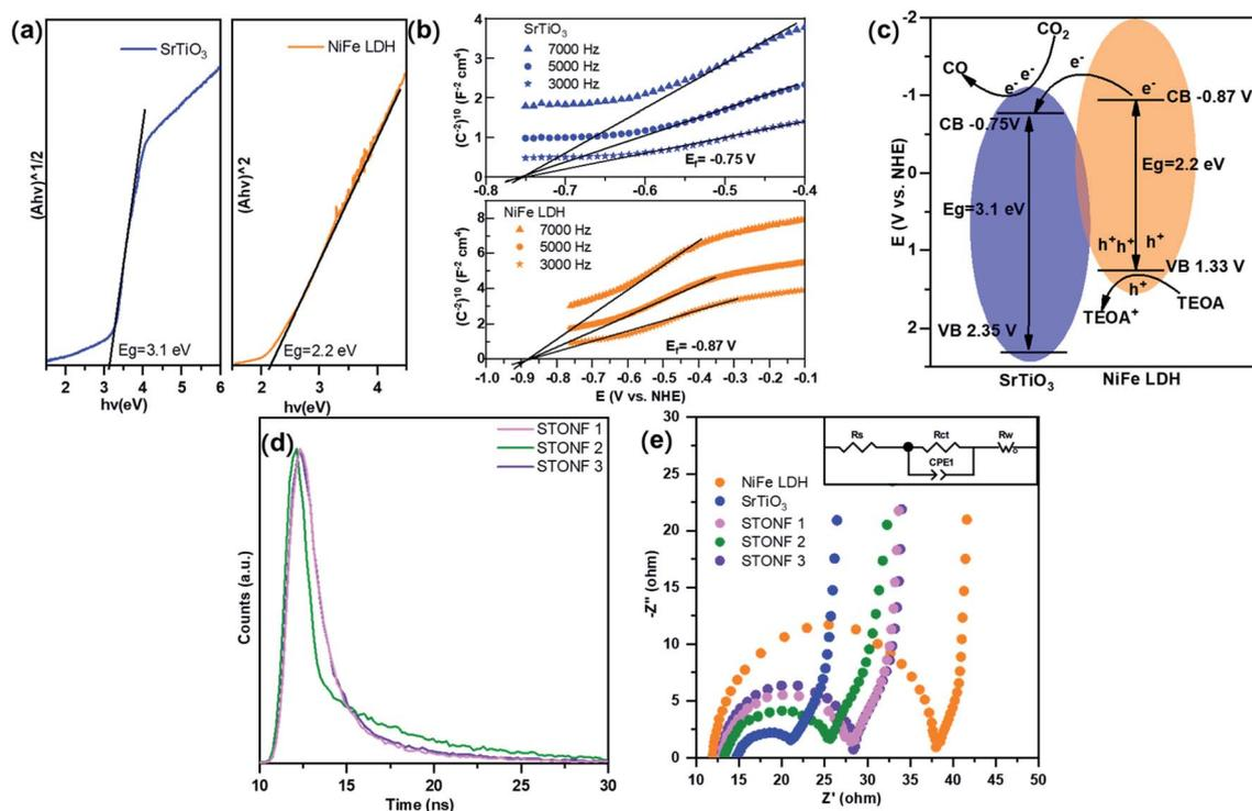
Fig. 4 (a) Tauc plots and (b) Mott–Schottky plots of SrTiO<sub>3</sub> and NiFe LDH; (c) schematic illustration of band structure alignment in STONFs composites; (d) transient PL decays and (e) Nyquist plots of as-prepared catalysts.
