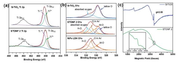
Fig. 5 XPS spectra of (a) the Ti 2p region and (b) O 1s region for as-prepared catalysts; (c) EPR signals of SrTiO₃ and STONF 2.
