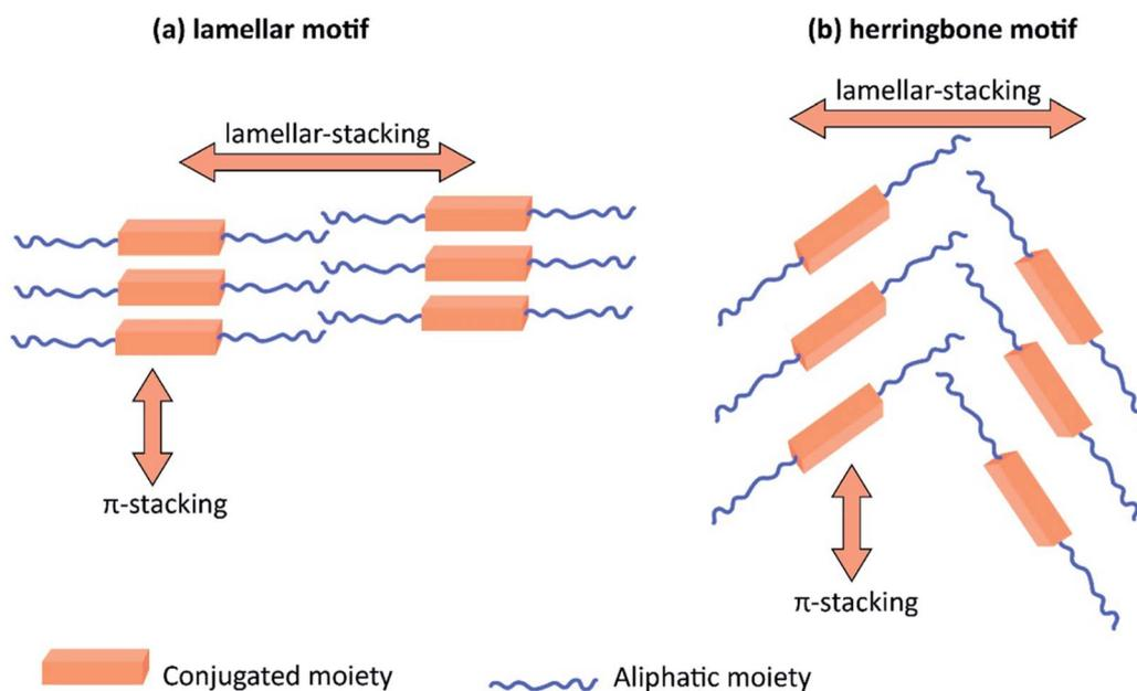
**Scheme 5** The  $\pi$ - and lamellar stacking for a series of naphthalene tetracarboxylic diimide (R-NDI) crystals giving rise to the lamellar motif and herringbone motif depending on the size of the aliphatic hydrocarbon moiety. This figure has been reproduced from ref. 73 with permission from ACS Omega, copyright 2018.
