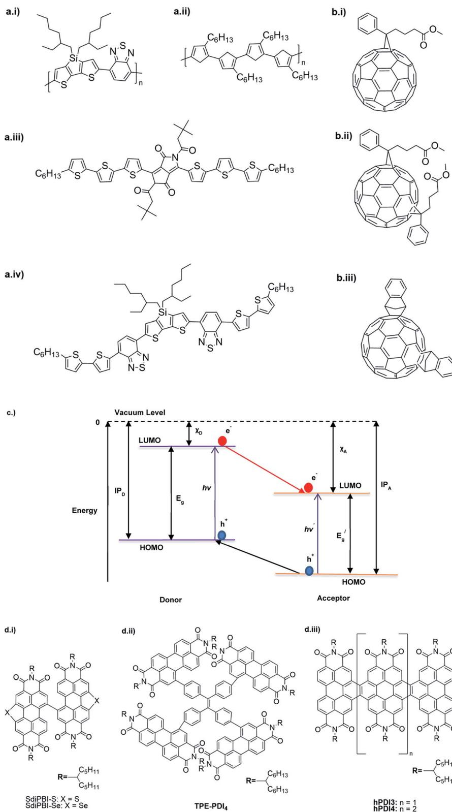
**Fig. 8** Commonly used (a) donor polymers (b) acceptor molecules both capable of absorbing radiation to generate electron–hole pairs, (c) energy level diagram showing electron–hole pair formation and separation in the donor–acceptor systems and (d) novel non-fullerene acceptor developed for use in organic solar cells. This figure has been reproduced from ref. 78 with open access permission from *Progress in Polymer Science*, copyright 2013.
