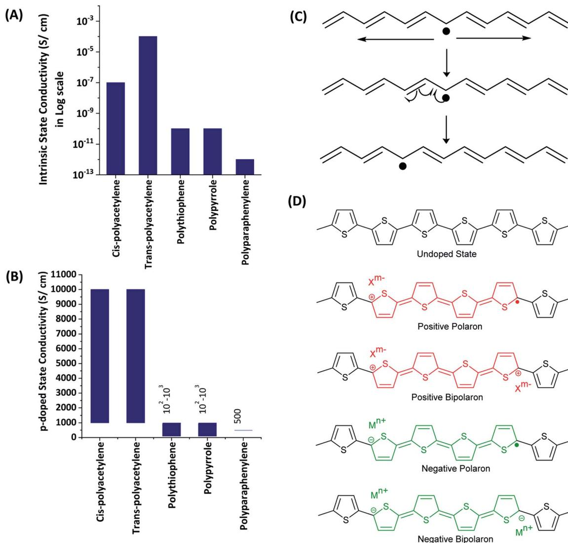
Fig. 2 Conductivities of some electronically conducting polymers in the (A) intrinsic and, (B) p-doped states. (C) Illustration of the native solitons of *trans*-polyacetylene. (D) Charge carriers such as positive, negative polarons and positive, negative bipolarons of polythiophene.
