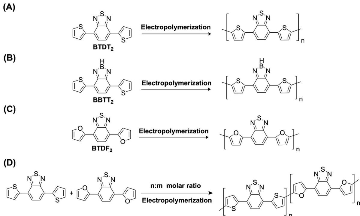
**Scheme 4** Electropolymerization reactions of (A) 4,7-dithiophen-2-yl-2,1,3-benzothiadiazole (BTDT<sub>2</sub>), (B) 2,5-di(thien-2-yl)-benzodiazaborole (BBTT<sub>2</sub>) (C) 4,7-difuran-2-yl-2,1,3-benzothiadiazole (BTDF<sub>2</sub>) and, (D) BTDT<sub>2</sub> and BTDF<sub>2</sub> mixtures in various molar ratios such as 1 : 1, 1 : 2, 2 : 1, 2 : 5 and 5 : 2 etc. This figure has been reproduced from ref. 42 with permission from RSC *Journal of Material Chemistry C*, copyright 2019.
