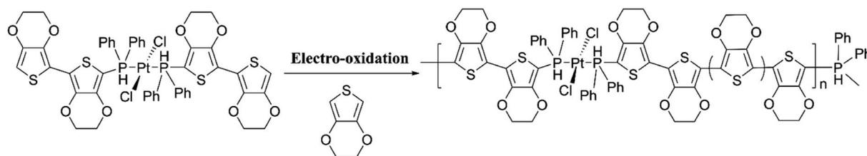
**Scheme 3** Electropolymerization of diphenyl(2,2',3,3'-tetrahydro-[5,5'-bithieno[3,4-*b*][1,4]dioxin]-7-yl)phosphane ( $\text{Ph}_2\text{P}[\text{bis-EDOT}]$ ) complex (**7**) with ethylenedioxythiophene in  $x : 1$  molar ratio to yield the copolymer with the same numbers of monomer units in the blocks. This figure has been reproduced from ref. 48 with open access permission from ScienceDirect, copyright 2017.
