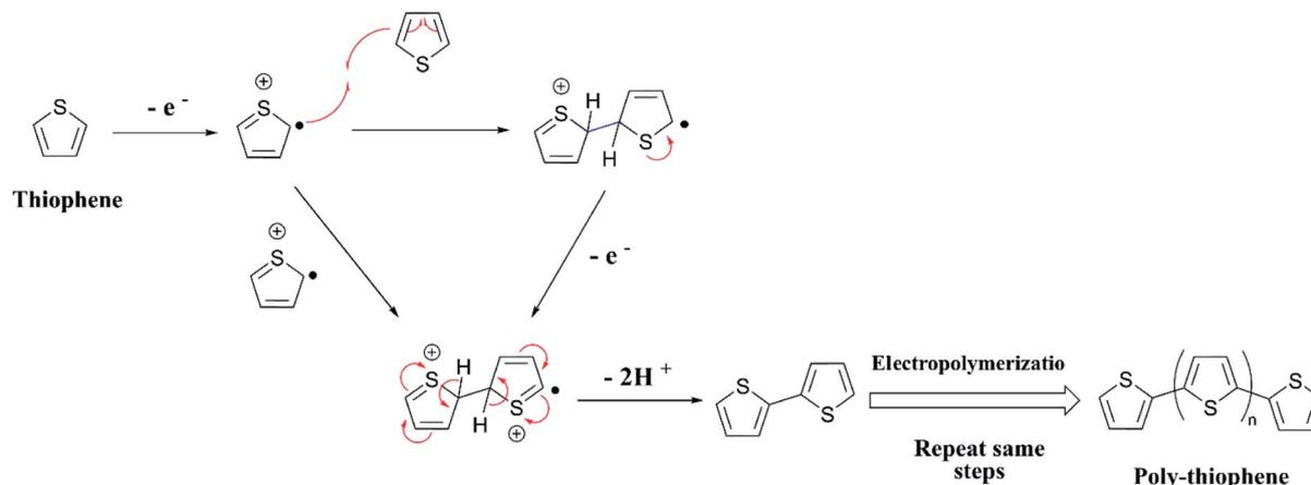
Scheme 1 Mechanism of the polymerization of thiophene.
