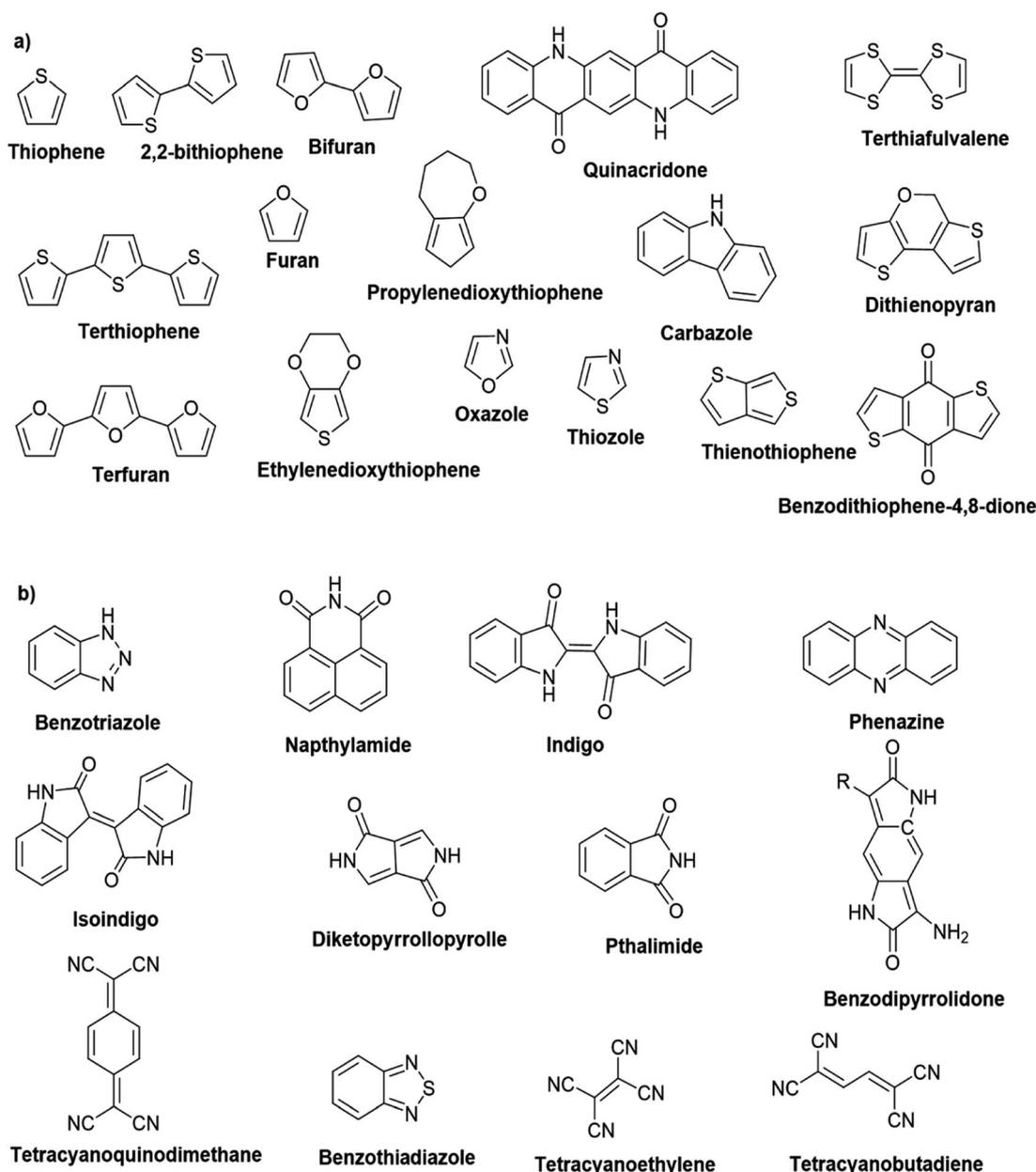
Fig. 5 Commonly used (a) electron donors (D) and, (b) electron acceptors (A) in making D-A type polymers.
