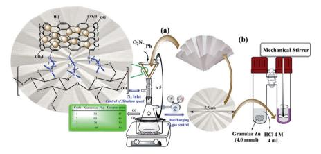
Scheme 2 Two setups for the (a) selective reduction of nitroarenes by the filtration method (method A), and (b) complete reduction of halogenated nitroarenes via the  $ex\ situ$  generated H<sub>2</sub> gas in a sealed tube (method B) on FP@Si@Pd/C catalytic filter paper.
