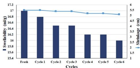
Fig. 7 Swellability and shrinkage measurements of FP@Si@Pd/C in MeOH : H<sub>2</sub>O (1 : 1, v/v) for 6 consecutive drying–wetting cycles.
