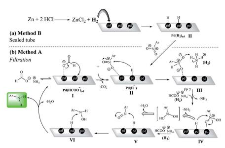
Scheme 5 Two plausible reaction mechanisms for the nitrobenzene reduction by (a) sealed (method B) and (b) filtration methods (method A).
