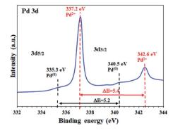
Fig. 3 High resolution XPS analysis (energy corrected, normalized) of Pd on activated carbon-immobilized cellulose filter paper (FP@Si@Pd/C).
