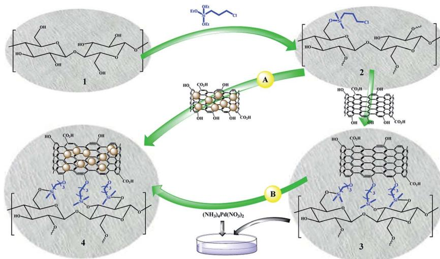
Scheme 3 General schematic view for the preparation of FP@Si@Pd/C catalytic filter paper (**4**) *via* two different routes.
