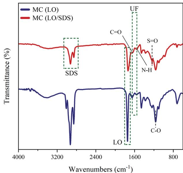
Fig. 5 FT-IR spectra of LO and LO/SDS microcapsules.
