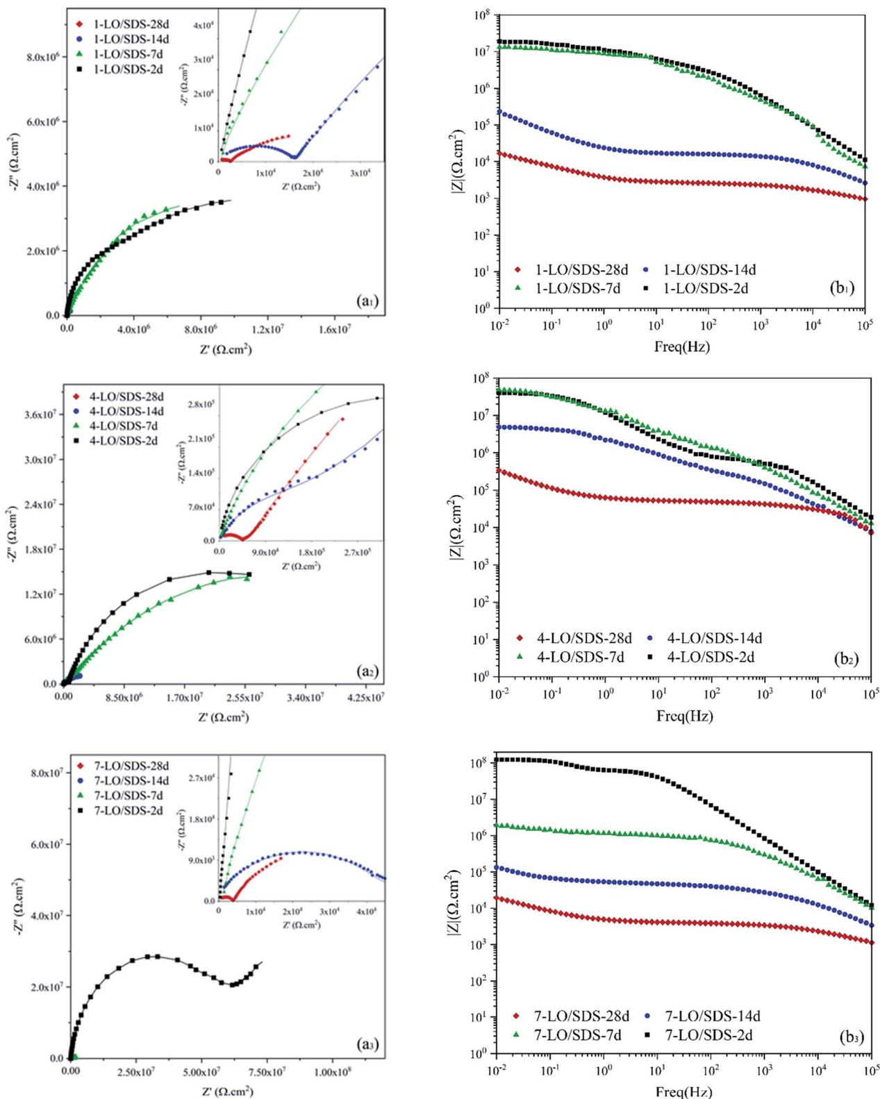
Fig. 14 (a) Nyquist and (b) Bode plots of scratched coating specimens loaded with different concentrations of LO/SDS microcapsules after various exposure times to 3.5 wt% NaCl.
