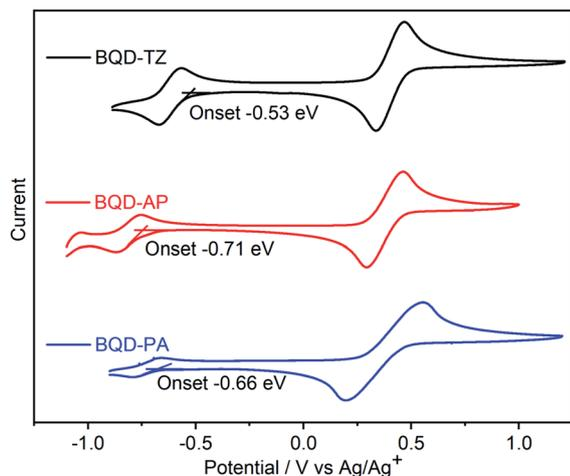
Fig. 2 The reduction curves of BQD-TZ, BQD-AP and BQD-PA in dichloromethane.
