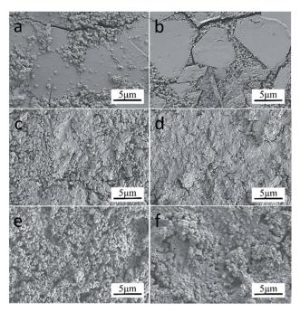
Fig. 8 SEM images of glass-ceramics treated at  $950\,^{\circ}$ C under different addition: (a) S1; (b) S2; (c) S3; (d) S4; (e) S5; (f) S6.
