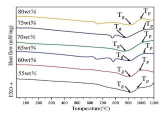
Fig. 2 DSC curves of glass-ceramics with different tailings.
