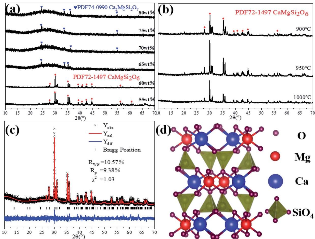
Fig. 3 (a) XRD patterns of glass-ceramics treated at 950 °C with different additions, (b) XRD patterns of glass-ceramics with 60 wt% tailings addition at different heat treatment temperatures, (c) Rietveld refinement of X-ray diffraction pattern of glass-ceramics with 60 wt% tailings addition at 950 °C, and (d) crystal structure of the diopside phase ( $\text{CaMgSi}_2\text{O}_6$ ).
