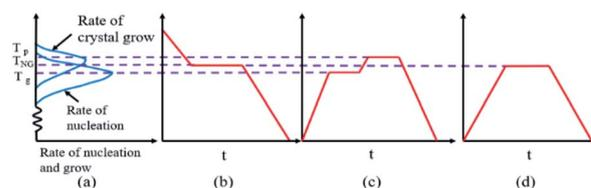
**Fig. 1** Heat treatment regime curve: (a) heat treatment temperature is determined by nucleation rate and crystal growth rate, (b) one-step direct cooling heat treatment, (c) nucleation and crystallization two-step heat treatment, and (d) nucleated crystallization one-step heat treatment.
