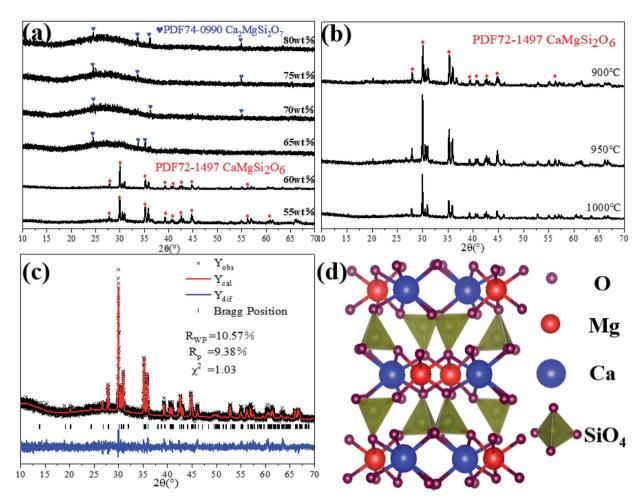
Fig. 3 (a) XRD patterns of glass-ceramics treated at 950  $^{\circ}$ C with different additions, (b) XRD patterns of glass-ceramics with 60 wt% tailings addition at different heat treatment temperatures, (c) Rietveld refinement of X-ray diffraction pattern of glass-ceramics with 60 wt% tailings addition at 950  $^{\circ}$ C, and (d) crystal structure of the diopside phase (CaMgSi<sub>2</sub>O<sub>6</sub>).
