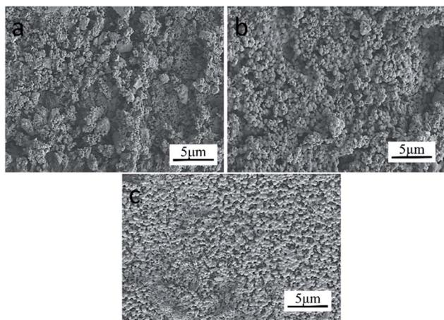
Fig. 9 SEM images of glass-ceramics with 60 wt% tailings addition at different heat treatment temperatures: (a) 900 °C, (b) 950 °C, and (c) 1000 °C.
