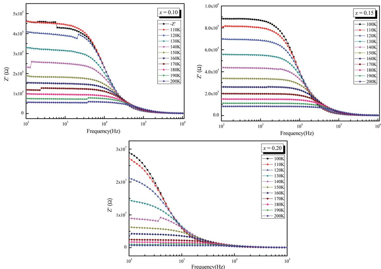
Fig. 6 Variation of real part of impedance ( $Z'$ ) as a function of frequency ( $\omega$ ) of  $\text{La}_{0.5}\text{Sm}_{0.2}\text{Sr}_{0.3}\text{Mn}_{1-x}\text{Cr}_x\text{O}_3$  ( $x = 0.10, 0.15$  and  $0.20$ ).
