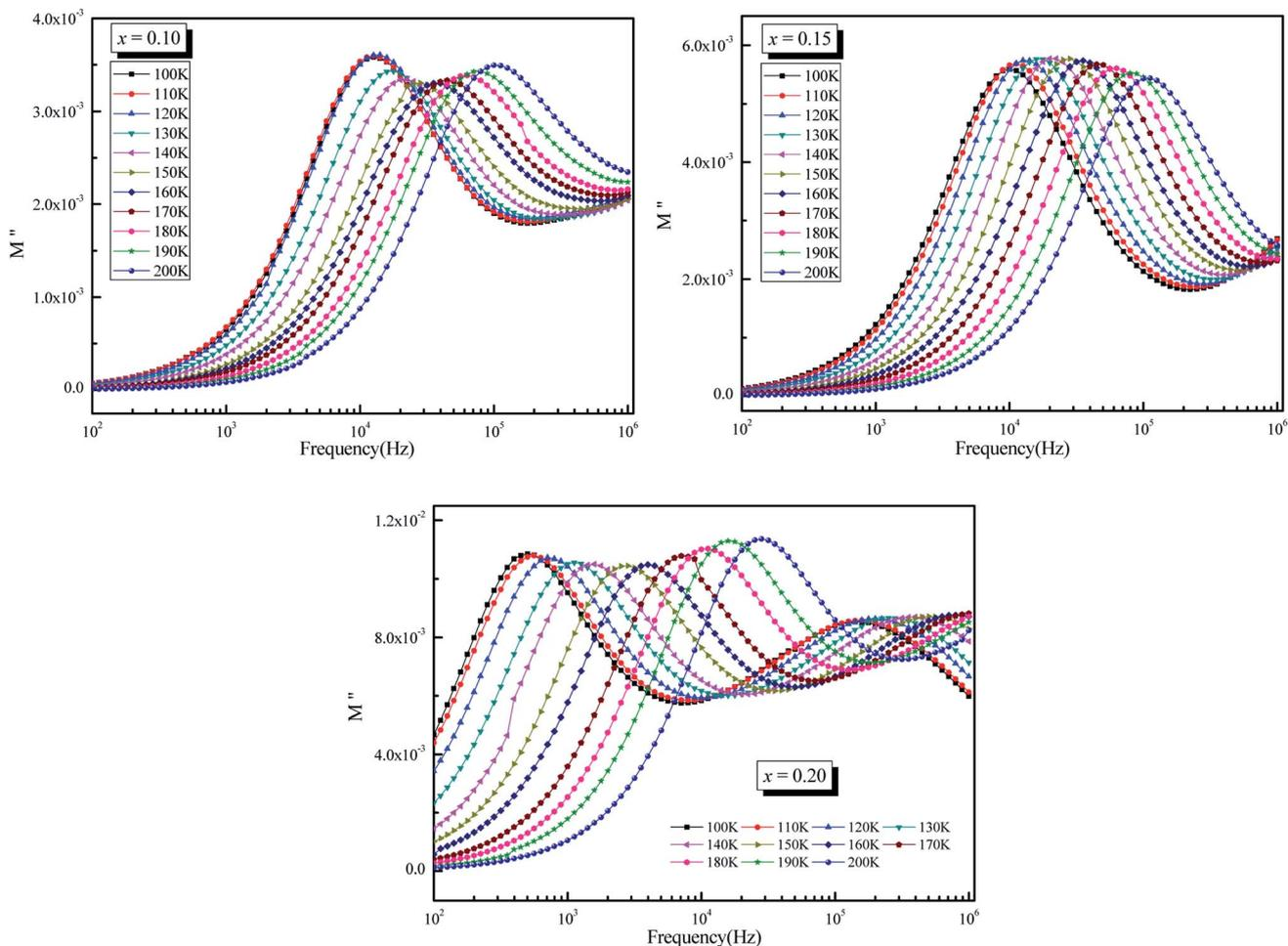
Fig. 11 Variation of imaginary part of modulus ( $M''$ ) as a function of frequency ( $\omega$ ) at different temperatures for  $\text{La}_{0.5}\text{Sm}_{0.2}\text{Sr}_{0.3}\text{Mn}_{1-x}\text{Cr}_x\text{O}_3$  ( $x = 0.10, 0.15$  and  $0.2$ ).
