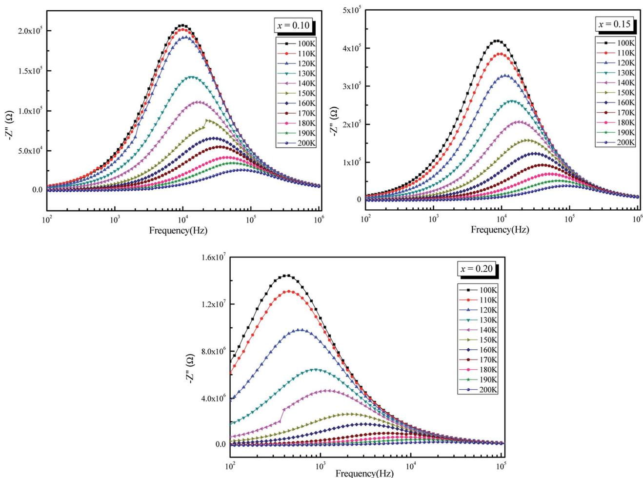
Fig. 7 Variation of imaginary part of impedance ( $-Z''$ ) as a function of frequency ( $\omega$ ) of  $\text{La}_{0.5}\text{Sm}_{0.2}\text{Sr}_{0.3}\text{Mn}_{1-x}\text{Cr}_x\text{O}_3$  ( $x = 0.10, 0.15$  and  $0.20$ ).
