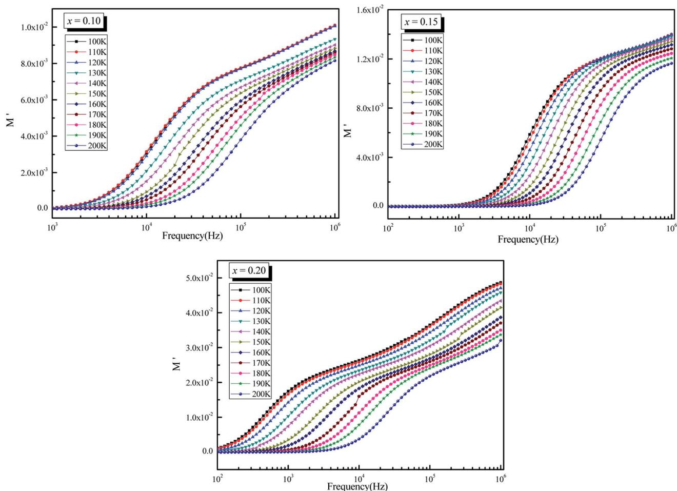
Fig. 10 Variation of real part of modulus ( $M'$ ) as a function of frequency ( $\omega$ ) at different temperatures for  $\text{La}_{0.5}\text{Sm}_{0.2}\text{Sr}_{0.3}\text{Mn}_{1-x}\text{Cr}_x\text{O}_3$  ( $x = 0.10, 0.15$  and  $0.2$ ).
