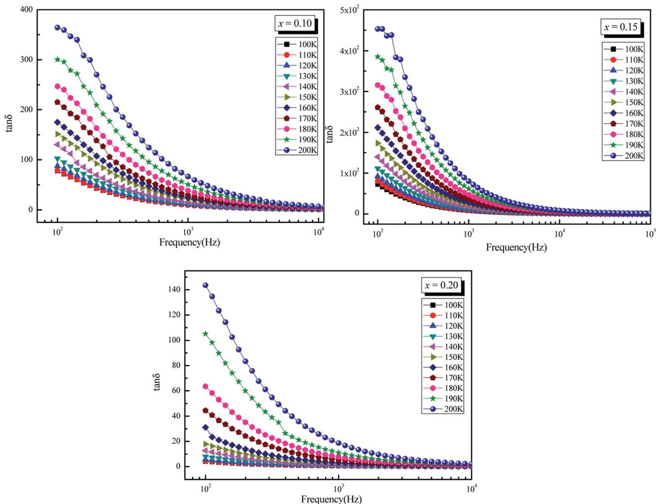
Fig. 5 Dielectric loss tangent ( $\tan \delta$ ) versus Logarithm of ( $\omega$ ) at different temperatures for  $\text{La}_{0.5}\text{Sm}_{0.2}\text{Sr}_{0.3}\text{Mn}_{1-x}\text{Cr}_x\text{O}_3$  ( $x = 0.10, 0.15$  and  $0.20$ ).
