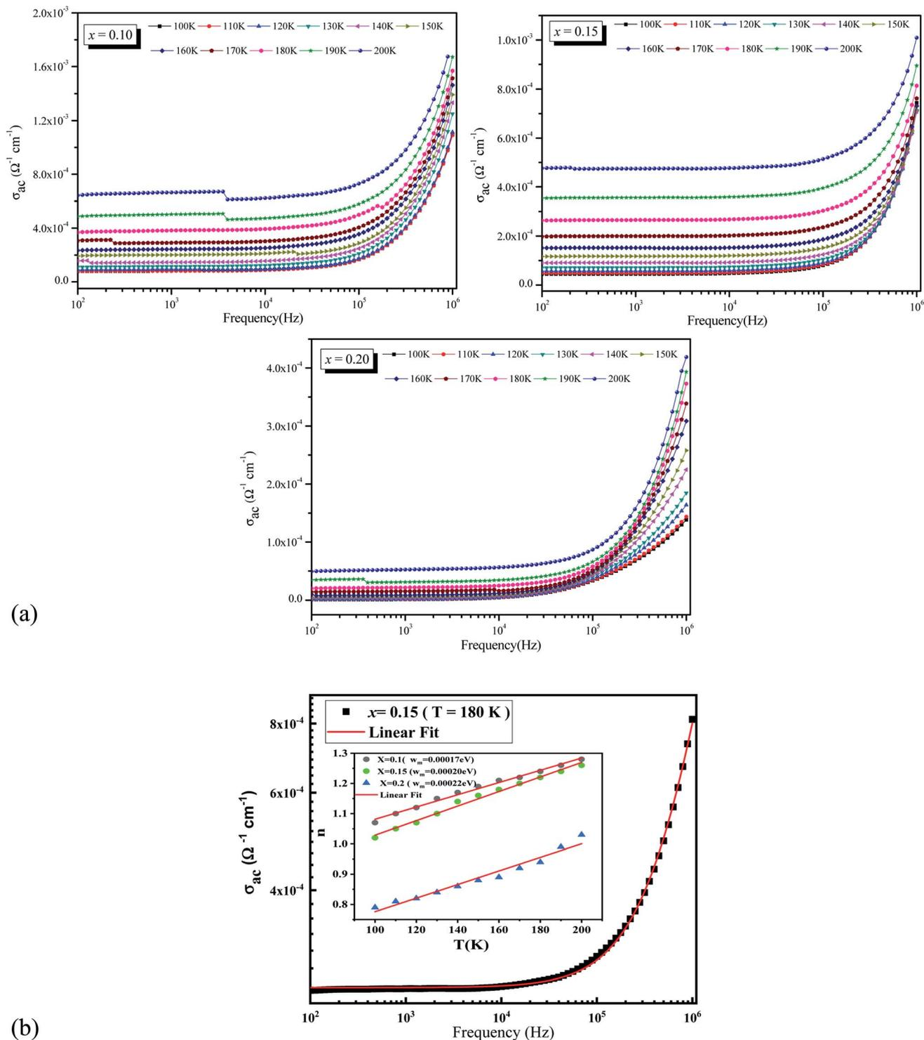
Fig. 2 (a) Frequency dependence of ac conductivity ( $\sigma_{ac}$ ) at various temperatures of  $\text{La}_{0.5}\text{Sm}_{0.2}\text{Sr}_{0.3}\text{Mn}_{1-x}\text{Cr}_x\text{O}_3$  ( $x = 0.10, 0.15$  and  $0.20$ ). (b) Typical example (conductivity vs. frequency at  $T = 180 \text{ K}$  for  $x = 0.15$ ) fitted using the universal Jonscher power law. The inset shows the variation of the exponent  $n$  vs. temperature for ( $x = 0.10, 0.15$  and  $0.20$ ).
