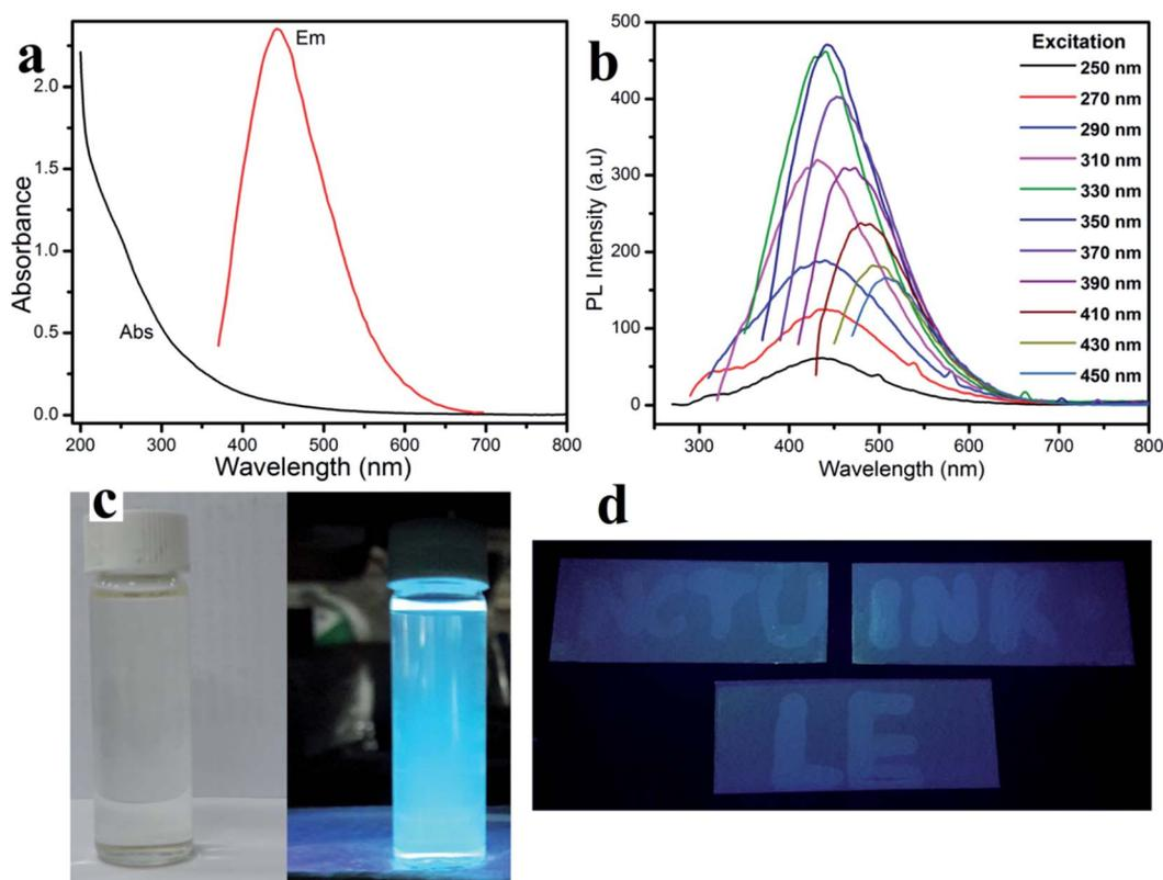
Fig. 2 (a) UV-vis absorption spectra and emission spectra at an excitation wavelength of 350 nm, (b) fluorescent spectra of the CDs, (c) photograph of the CDs under daylight (left) and 365 nm UV light (right) and (d) photograph of QD ink on an aluminum thin-layer chromatography (TCL) plate.
