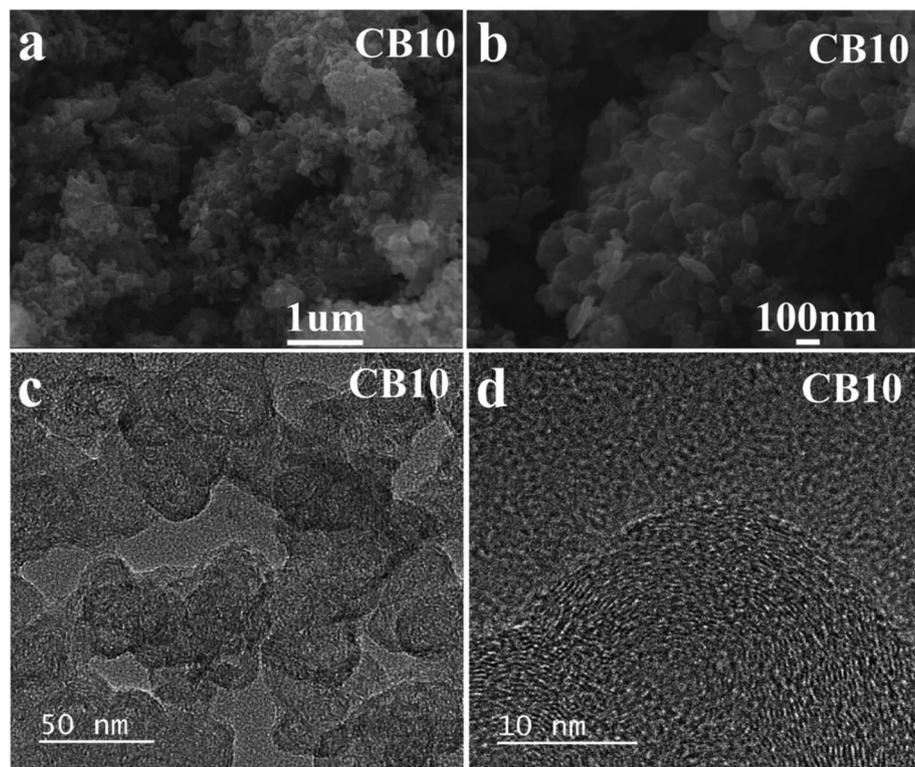
Fig. 6 (a and b) SEM and (c and d) TEM images of porous carbon CB10 at various magnifications.
