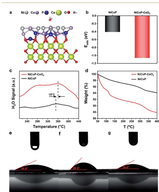
Fig. 5 Optimized adsorption structures of NiCoP–CeO<sub>2</sub> (a); adsorption energies of H<sub>2</sub>O on NiCoP and NiCoP–CeO<sub>2</sub> (b); H<sub>2</sub>O TPD spectra of NiCoP and NiCoP–CeO<sub>2</sub> (c); thermogravimetric analysis of NiCoP and NiCoP–CeO<sub>2</sub> (d); wetting-ability testing of (e) NiCo-LDHs, (f) NiCoP and (g) NiCoP–CeO<sub>2</sub>.
