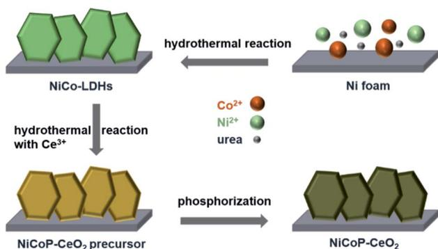
Fig. 1 The synthetic scheme of the NiCoP-CeO<sub>2</sub> electrode.
