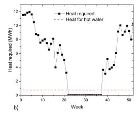
Fig. 3 The main parameters required for the system design: (a) the energy availability from the solar panels and the electricity requirements of the building, (b) the heat required in the building in the form of ambient heat and hot sanitary water.
