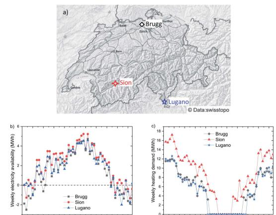
Fig. 6 Input data for the geographic sensitivity analysis: (a) the geographical positioning of the locations selected for the sensitivity analysis, (b) the electricity availability profile over the year for the three locations (negative numbers indicate an excess demand), (c) the heating demand over the year for the three locations.
