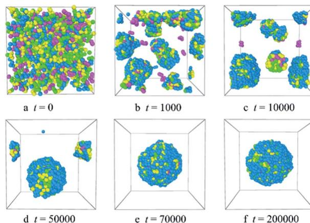
Fig. 5 Representative morphologies of Dtx-loaded PLGA<sub>3</sub>-*b*-PEG<sub>7</sub>-*b*-PLGA<sub>3</sub> micelles at different simulation times. The green, yellow and blue spheres represent beads L, G, and E respectively, and the pink spheres represent beads D1, D2, and D3 of the Dtx drug.
