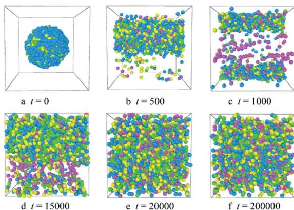
Fig. 9 Representative morphologies of Dtx-loaded PLGA<sub>3</sub>-*b*-PEG<sub>7</sub>-*b*-PLGA<sub>3</sub> micelles at different simulation times with shear rate 3.5. The green, yellow and blue spheres represent beads L, G, and E respectively, and the pink spheres represent beads D1, D2, and D3 of the Dtx drug.
