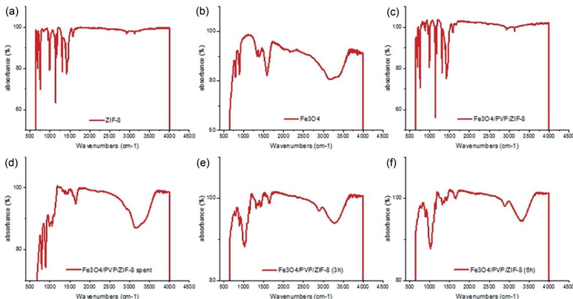
Fig. 2 FTIR spectra of: (a) ZIF-8; (b) Fe<sub>3</sub>O<sub>4</sub> nanoparticles; (c) core-shell Fe<sub>3</sub>O<sub>4</sub>/PVP/ZIF-8 nanostructure; (d) spent core-shell Fe<sub>3</sub>O<sub>4</sub>/PVP/ZIF-8 nanostructure; (e) core-shell Fe<sub>3</sub>O<sub>4</sub>/PVP/ZIF-8 nanostructure at pH = 2 for 3 h; (f) core-shell Fe<sub>3</sub>O<sub>4</sub>/PVP/ZIF-8 nanostructure at pH = 2 for 6 h.
