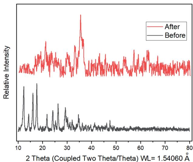
**Fig. 5** XRD patterns of core-shell Fe<sub>3</sub>O<sub>4</sub>/PVP/ZIF-8 nanostructure adsorbent; before Fosfomycin adsorption (lower gray line), after Fosfomycin adsorption at pH 2 for 6 h (upper red line).
