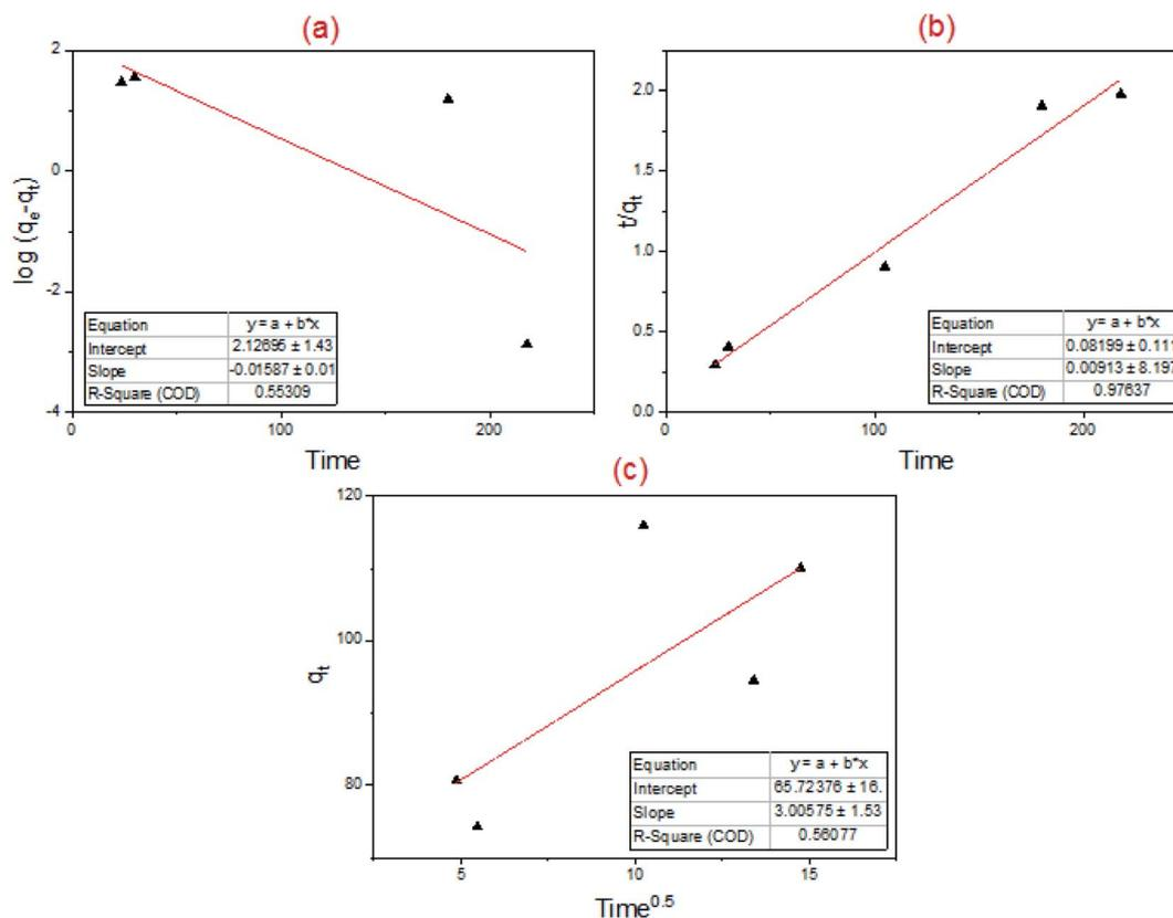
Fig. 13 Kinetics models: (a) pseudo 1<sup>st</sup> order model; (b) pseudo 2<sup>nd</sup> order model; (c) intra-particle diffusion kinetic model.
