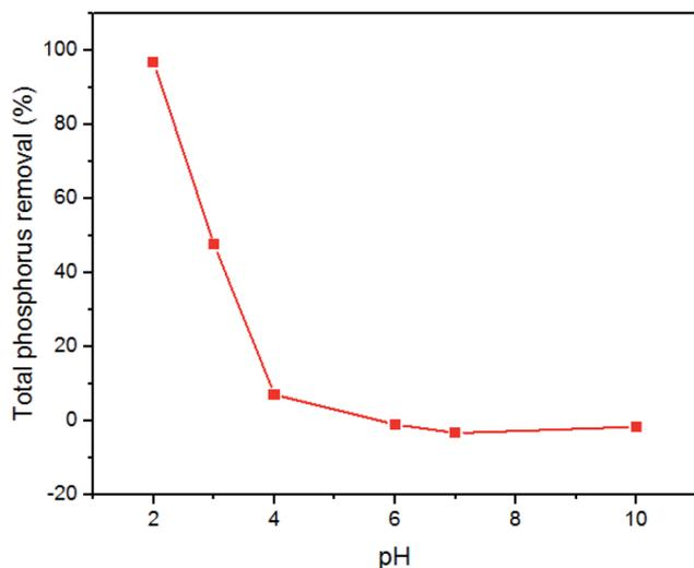
Fig. 7 pH vs. % TP removal. Conditions: 0.3 g/100 mL, 30 mg-P L<sup>-1</sup> initial concentration of TP, 200 rpm, 75 min, and 25 °C.
