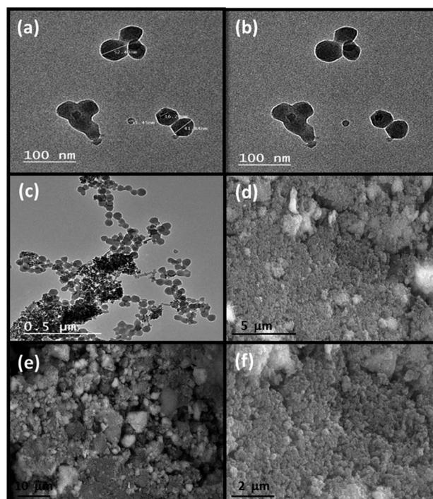
Fig. 3 (a-c) TEM images of core-shell Fe<sub>3</sub>O<sub>4</sub>/PVP/ZIF-8 nanostructure adsorbent at different magnifications demonstrating the successful formation of core-shell structures; (d-f) SEM images of core-shell Fe<sub>3</sub>O<sub>4</sub>/PVP/ZIF-8 nanostructure adsorbent at different magnifications.
