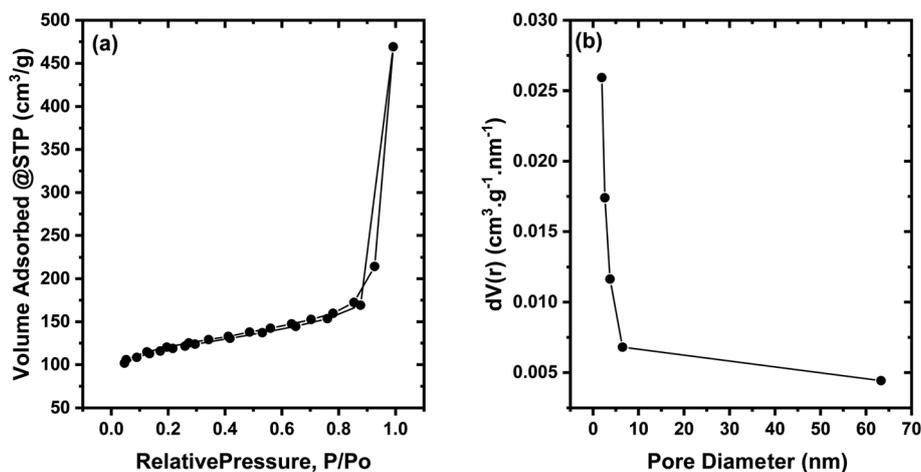
**Fig. 6** (a) The N<sub>2</sub> gas adsorption–desorption measurements of core-shell Fe<sub>3</sub>O<sub>4</sub>/PVP/ZIF-8 nanostructure adsorbent; (b) pore size distribution adsorption as estimated by BJH theory.
