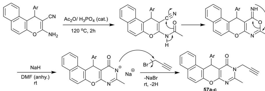
Scheme 33 Synthesis of naphtha-pyranopyrimidinones.
