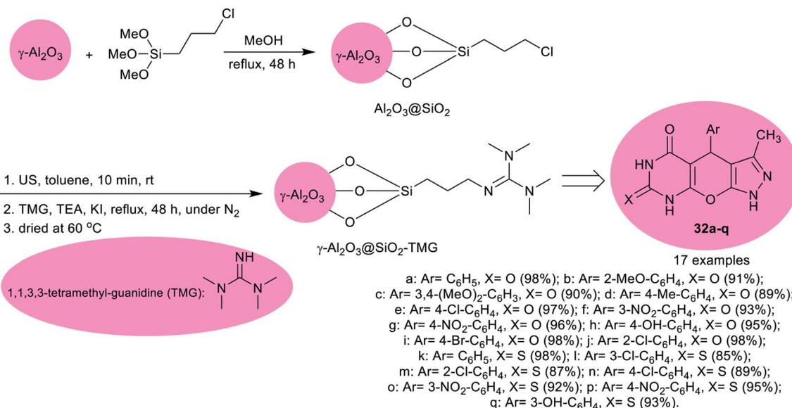
Scheme 21 Synthesis of  $\gamma$ -Al<sub>2</sub>O<sub>3</sub>@silane-TMG nano-catalyst for the synthesis of pyrazolo-pyranopyrimidinones.
