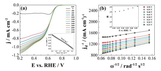
Fig. 5 LSV curves in O<sub>2</sub>-saturated 1 M KOH at different rotation rates with Tafel plot at 1800 rpm in inset (a) and corresponding Koutecky–Levich plots at different potentials with the number of exchanged electrons in inset (b).
