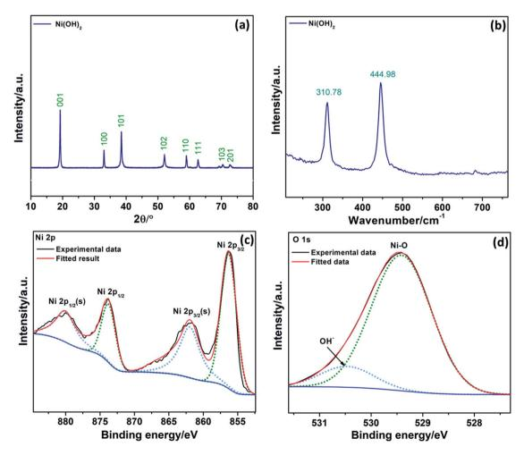
Fig. 3 XRD (a) and Raman spectra (b) of Ni(OH)<sub>2</sub>. XPS spectra of Ni 2p (c) and O 1s (d) for Ni(OH)<sub>2</sub>
