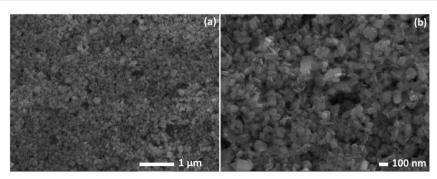
Fig. 1 SEM images of Ni(OH)<sub>2</sub> at different magnifications (a and b).
