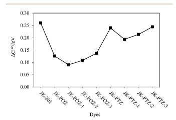
Fig. 8 Variations of the driving force of regeneration ( $\Delta G^{\text{reg}}$ ) of the reference and designed dyes.
