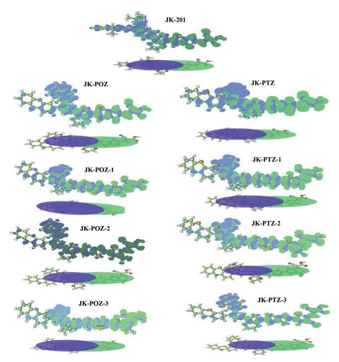
Fig. 6 The calculated charge density differences between the ground and excited states of the reference and designed dyes. Green and blue regions correspond to positive and negative regions, respectively; they represent an increase and decrease in electron density due to the excitation, respectively.
