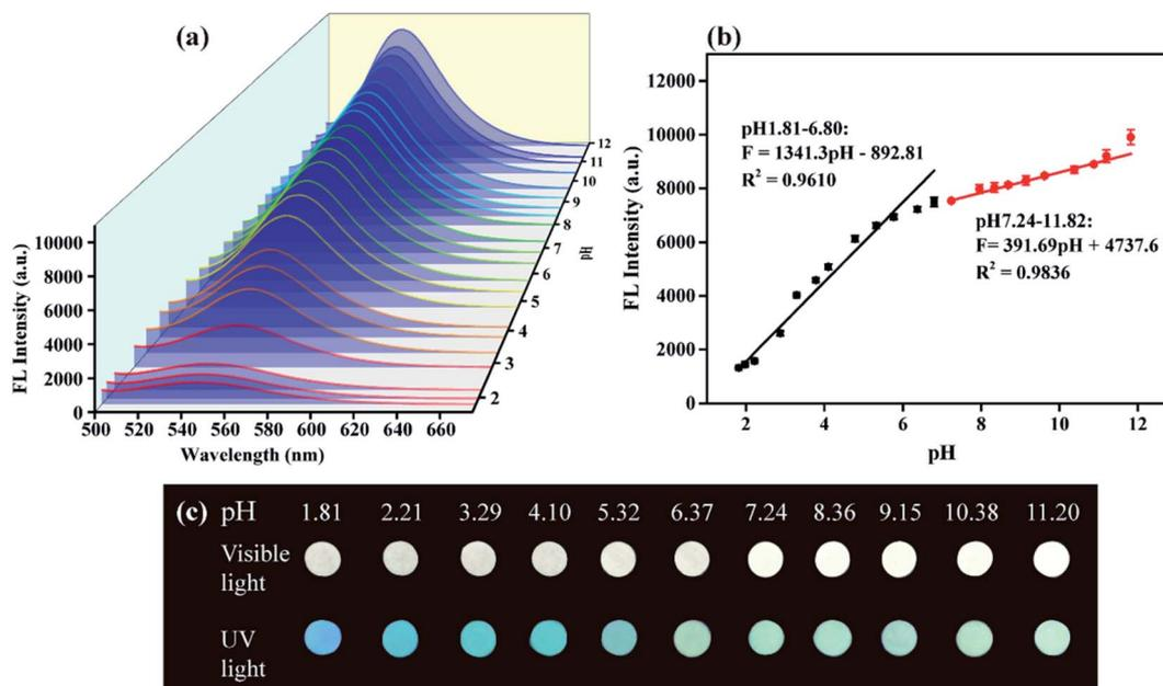
Fig. 6 (a) 3D FL emission spectra of the fluorescent sensor at various pH values. (b) The linear relationship between FL intensity and various pH values. (c) Photographs of NCDs-LM-based test paper of different pH values under ultraviolet light (365 nm).
