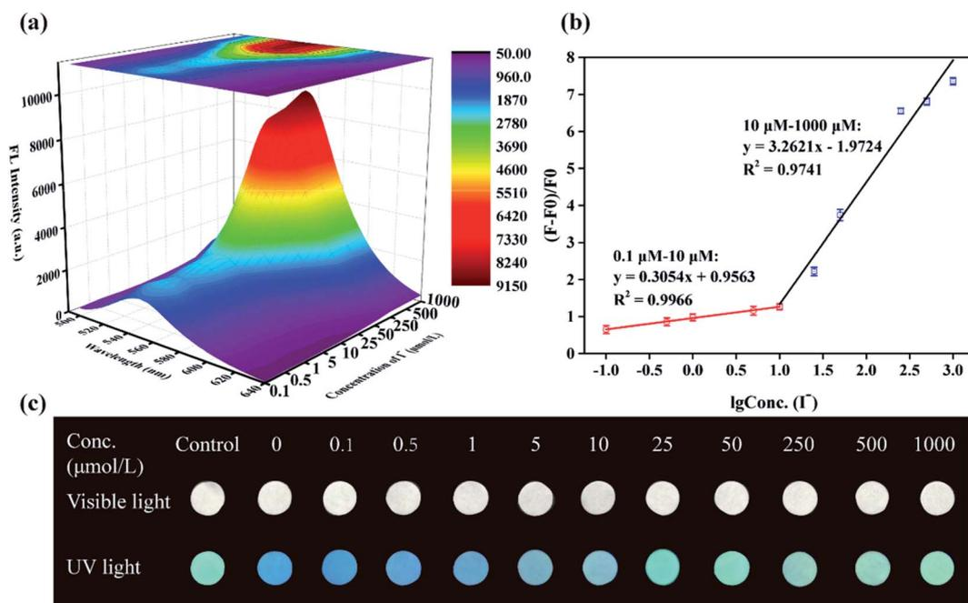
Fig. 5 (a) 3D FL emission spectra of the fluorescent sensor in the presence of different concentrations of  $I^-$ . (b) The linear relationship between  $(F_0-F)/F_0$  and the concentration of  $I^-$ . (c) Photographs of NCDs-LM-based test paper: only NCDs-LM (control), NCDs-LM- $Hg^{2+}$ (0), and the mixed solution containing NCDs-LM- $Hg^{2+}$  and different concentrations of  $I^-$  under ultraviolet light (365 nm).
