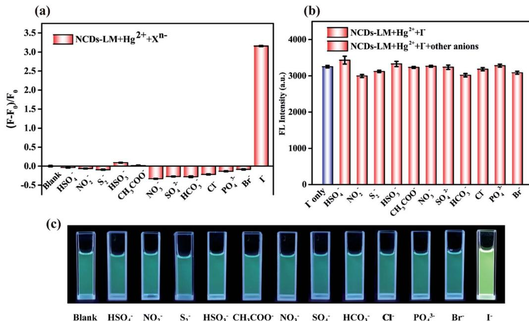
Fig. 4 (a) Selectivity of NCDs-LM-based sensor towards  $I^-$  with other interferents. (b) Interference experiments of NCDs-LM-based sensor towards  $I^-$  (blue bars) and other interference ions (red bars). (c) The photograph of NCDs-LM-based sensor under a 365 nm UV lamp after adding  $I^-$  and other interferents.
