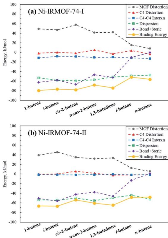
Fig. 3 Decomposition of  $C_4$  binding energies to the Ni-IRMOF-74 structures. The individual contributing terms to the binding energies are defined in eqn (2)–(6) in the ESI,<sup>†</sup> and sum to the total binding energy (also included in the figure).
