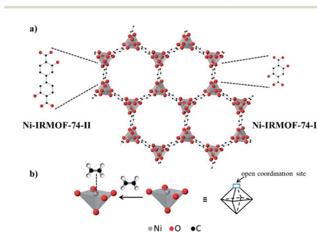
**Fig. 1** (a) Schematic structure of two isorecticular Ni-MOF-74 structures – smaller pore, Ni-IRMOF-74-I and bigger pore (larger linker), Ni-IRMOF-74-II and (b) open metal site in the structure, and its binding to an ethylene molecule. The framework structure is taken from ref. 1.
