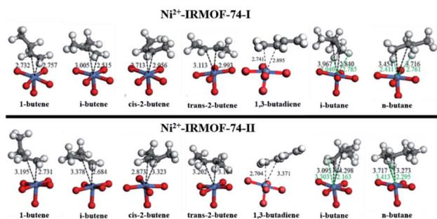
Fig. 2 Adsorbed geometries of C<sub>4</sub> isomers on Ni-IRMOF-74-I (top) and Ni-IRMOF-74-II (bottom). Black dotted lines represent Ni–C distances, while green dotted lines represent Ni–H distances. Distances are labelled in Angstrom.
