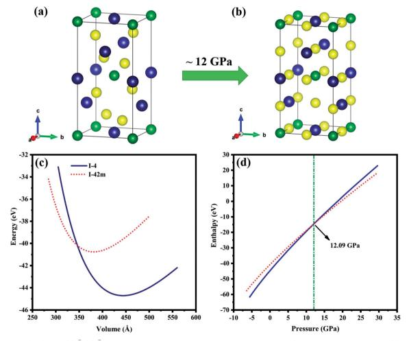
Fig. 1 Unit cell of  $ZnGa_2Te_4$  (a)  $I\overline{4}$ , (b)  $I\overline{4}2m$  phases. The green, blue and yellow balls represent Zn, Ga and Te atoms respectively. (c) BM-EOS fit, (d) enthalpy as a function of pressure.
