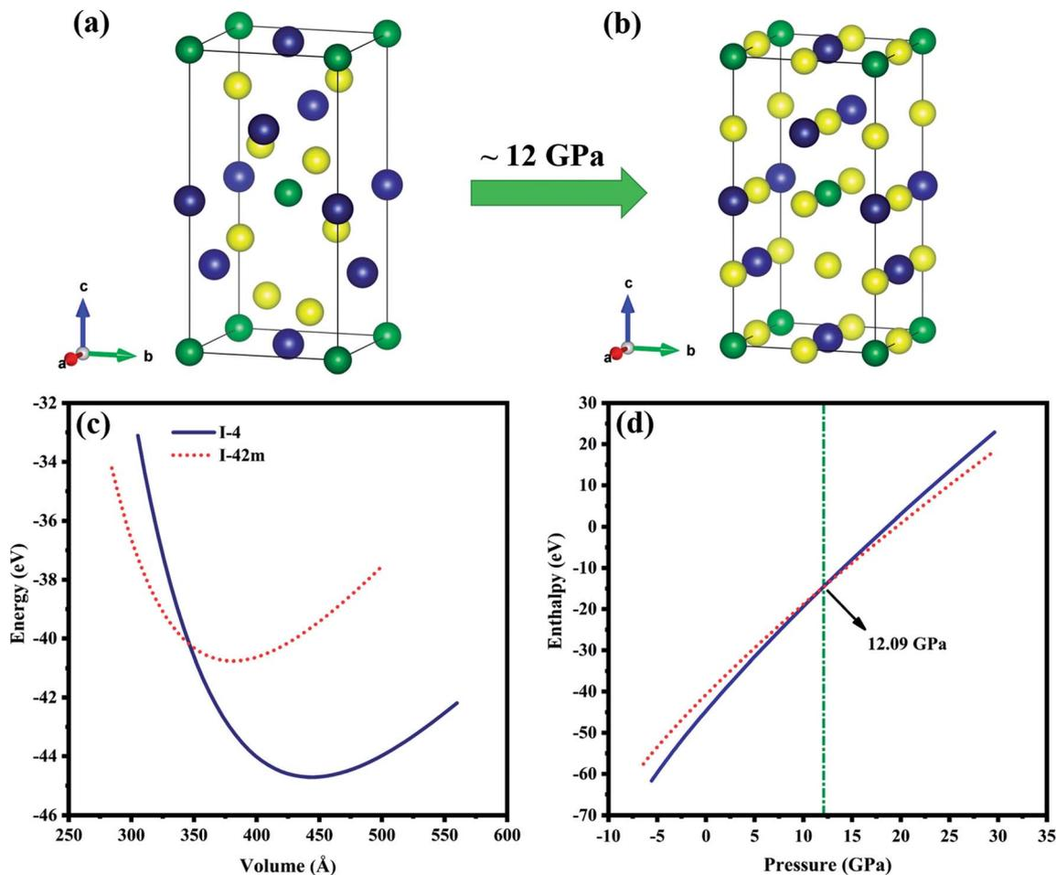
Fig. 1 Unit cell of  $\text{ZnGa}_2\text{Te}_4$  (a)  $I\bar{4}$ , (b)  $I\bar{4}2m$  phases. The green, blue and yellow balls represent Zn, Ga and Te atoms respectively. (c) BM-EOS fit, (d) enthalpy as a function of pressure.
