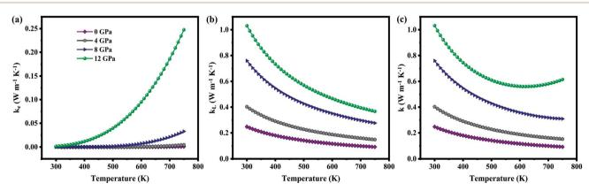
Fig. 8 (a) Electronic, (b) lattice, (c) total thermal conductivity as a function of temperature at various pressure.
