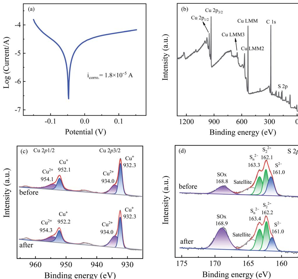
Fig. 6 (a) Tafel scans of  $\text{Cu}_2\text{S}$  electrode, (b) XPS survey spectrum, (c) Cu 2p and (d) S 2p XPS spectra before and after use in the  $\text{Cu}_2\text{S}$ /sulfite process. Experimental conditions: [sulfite] =  $500 \mu\text{M}$ ,  $[\text{Cu}_2\text{S}] = 0.025 \text{ g L}^{-1}$ , [iohexol]<sub>0</sub> =  $10 \mu\text{M}$ , pH = 8.0.
