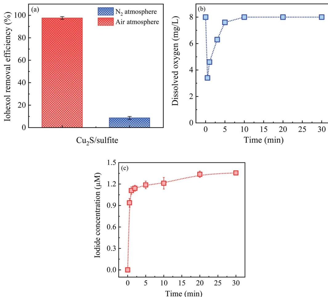
Fig. 5 (a) iohexol abatement under aerobic and anaerobic conditions, (b) variation of dissolved oxygen concentration in the Cu $_2$ S/sulfite process and (c) iodide release in the Cu $_2$ S/sulfite process. Experimental conditions: [sulfite] = 500  $\mu\text{M}$ , [Cu $_2$ S] = 0.025 g L $^{-1}$ , [iohexol] $_0$  = 10  $\mu\text{M}$ , pH = 8.0.
