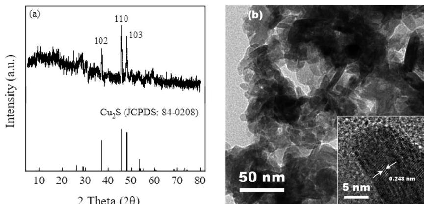
Fig. 1 (a) XRD pattern and (b) TEM images of  $\text{Cu}_2\text{S}$ .
