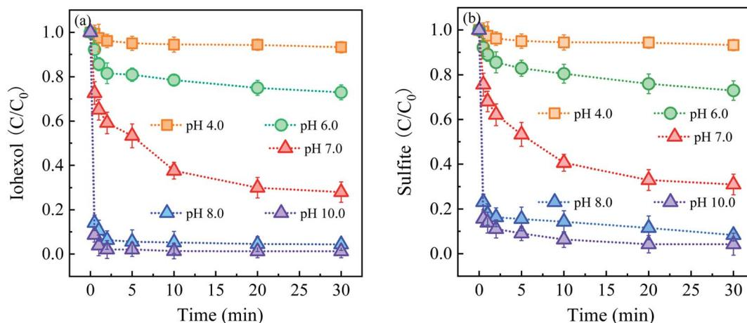
Fig. 3 (a) Effect of solution pH on iohexol abatement and (b) sulfite decay in the  $\text{Cu}_2\text{S/sulfite}$  process. Experimental conditions:  $[\text{sulfite}] = 500 \mu\text{M}$ ,  $[\text{Cu}_2\text{S}] = 0.025 \text{ g L}^{-1}$ ,  $[\text{iohexol}]_0 = 10 \mu\text{M}$ .
