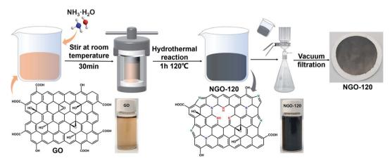
Fig. 1 Schematic diagram of NGO preparation.
