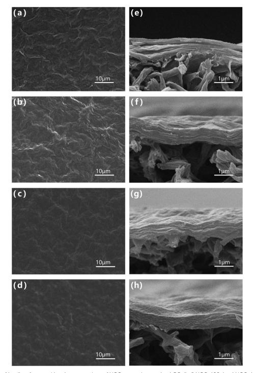
Fig. 2 SEM images of (a-d) surfaces and (e-g) cross sections of NGO-x membranes: (a, e) GO, (b, f) NGO-100, (c, g) NGO-120, (d, h) NGO-140.
