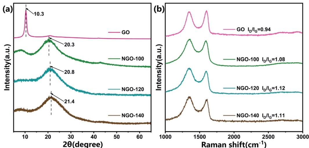
Fig. 3 (a) XRD patterns and (b) Raman spectra of NGO membranes.
