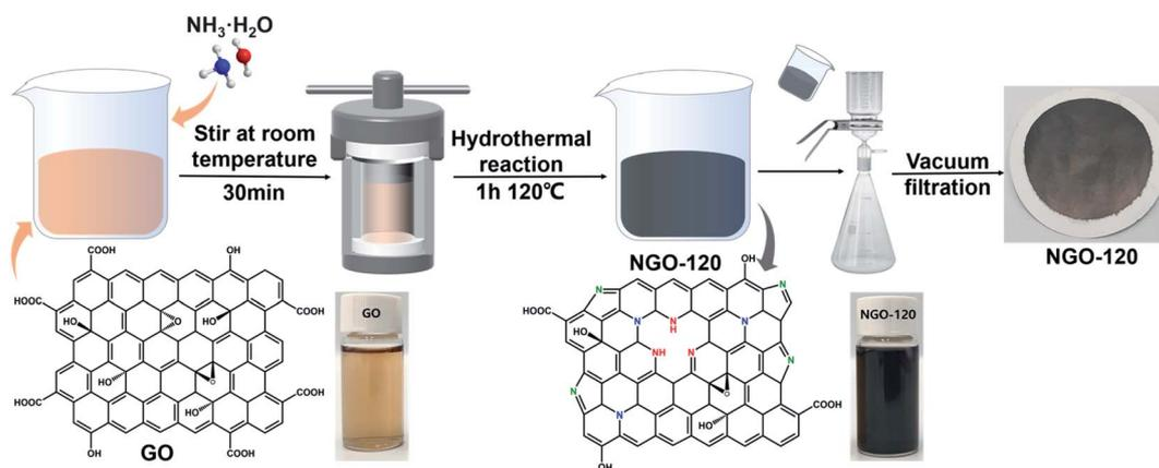
Fig. 1 Schematic diagram of NGO preparation.
