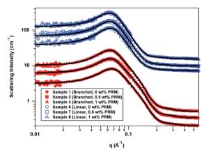
Fig. 1 SANS data overlays for branched-tail (red, solid symbols) and linear-tail (blue, empty symbols) mixed surfactant systems as a function of perfume concentration. The data sets are offset to improve clarity, with the 0.5 and 1 wt% perfume curves offset from the 0 wt% perfume curve by powers of 1.5, and the blue curves offset from the red curves by an additional factor of 20. The solid black lines are the model fits to the data.
