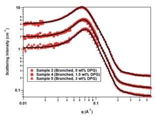
Fig. 2 SANS data overlays for the branched-tail mixed surfactant system as a function of DPG concentration. The data sets are offset to improve clarity, with the 1.5 and 3 wt% DPG curves offset from the 0 wt% DPG curve by powers of 2/3. The solid black lines are the model fits to the data. Location of perfume accord in micelles.
