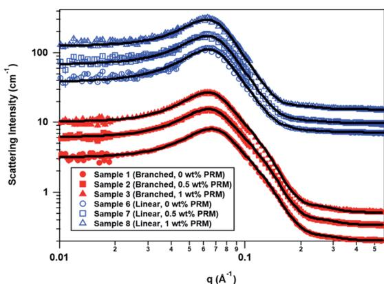
**Fig. 1** SANS data overlays for branched-tail (red, solid symbols) and linear-tail (blue, empty symbols) mixed surfactant systems as a function of perfume concentration. The data sets are offset to improve clarity, with the 0.5 and 1 wt% perfume curves offset from the 0 wt% perfume curve by powers of 1.5, and the blue curves offset from the red curves by an additional factor of 20. The solid black lines are the model fits to the data.
