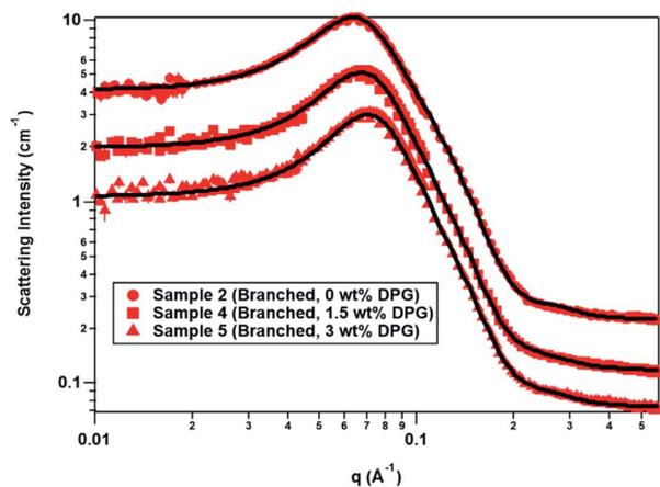
**Fig. 2** SANS data overlays for the branched-tail mixed surfactant system as a function of DPG concentration. The data sets are offset to improve clarity, with the 1.5 and 3 wt% DPG curves offset from the 0 wt% DPG curve by powers of 2/3. The solid black lines are the model fits to the data. Location of perfume accord in micelles.
