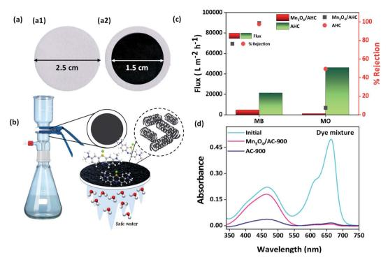
Fig. 4 Photographs of (a1) Whatman filter paper (a2) filter paper after  $Mn_3O_4/AHC$  via vacuum filtration. (b) Lab-scale continuous flow filtration setup for organic contaminant removal. (c) Flux and rejection for AHC and  $Mn_3O_4/AHC$  for MB and MO dyes removal via continuous flow and (d) UV-Vis spectra for dye mixture (MB + MO) removal using the prepared materials.
