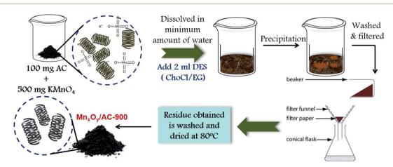
Fig. 1 Schematic for the room temperature synthesis of Mn<sub>3</sub>O<sub>4</sub>/AHC using deep eutectic solvent.
