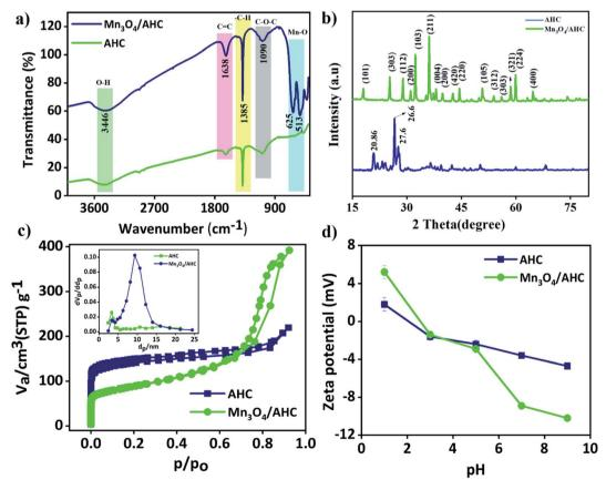
Fig. 3 (a) FTIR graph of TLCHs physically activated at 900 °C (AHC) and  $Mn_3O_4/AHC$  composite material, (b) diffraction peaks of XRD for AHC &  $Mn_3O_4/AHC$  samples. (c) BET surface area adsorption—desorption plot for the synthesized materials. Inset is a picture of pore size distribution in the as-synthesized material. (d) Surface charge trend of the synthesized materials.
