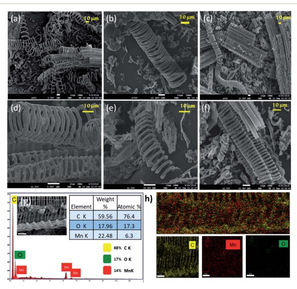
Fig. 2 FESEM micrographs of (a) and (d) HCFs obtained on solvothermal treatment. (b) and (e) HCFs physically activated at 900 °C (AHC). (c) and (f)  $Mn_3O_4$  functionalized HCFs ( $Mn_3O_4$ /AHC). (g) and (h) Elemental mapping of  $Mn_3O_4$  functionalized HCFs ( $Mn_3O_4$ /AHC).
