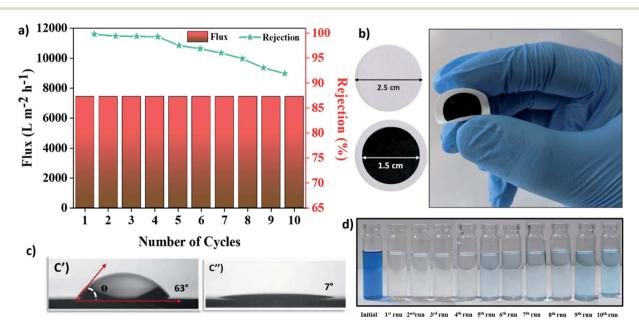
Fig. 6 (a) Regeneration study of  $Mn_3O_4/AHC$  for adsorption of MB dye. (b) Photograph of  $Mn_3O_4/AHC$  powder-based membrane. (c) Contact angle measurements for the prepared membranes. (c') AHC membrane, (c")  $Mn_3O_4/AHC$  membrane. (d) Digital photograph of permeates obtained during the recyclability study.
