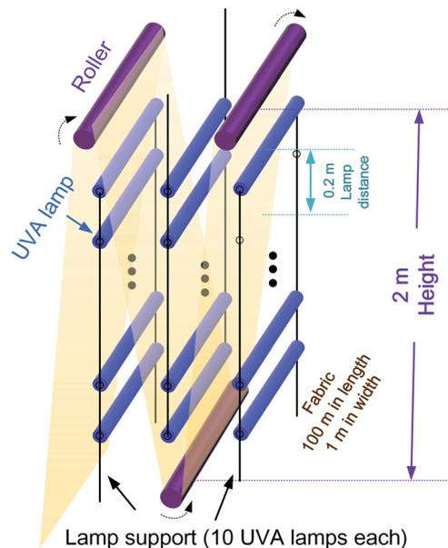
Fig. 9 Proposed continuous UVA-assisted scouring/bleaching process for fabric.
