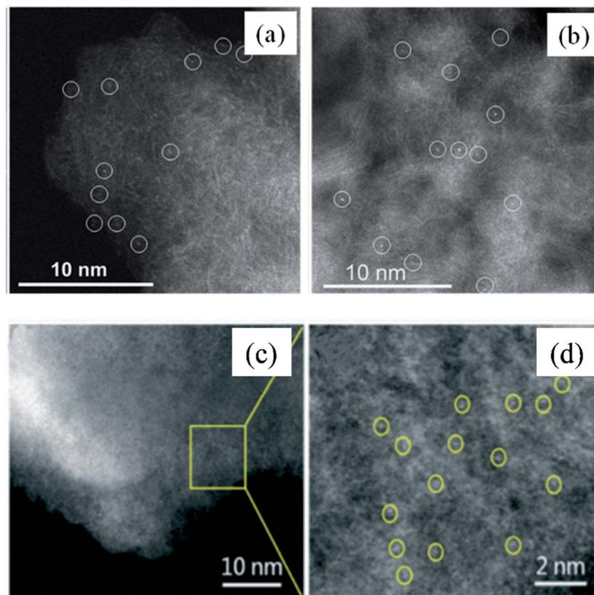
Fig. 3 HAADF-STEM image of Co-N-C catalyst prepared by the pyrolysis synthesis method (a and b) and Pd<sub>1</sub>/N-graphene catalyst prepared by the pyrolysis synthesis method (c and d). These figures have been adapted/reproduced from ref. 85 and 86 with permission from American Chemical Society and Royal Society of Chemistry, copyright 2015 and 2022.
