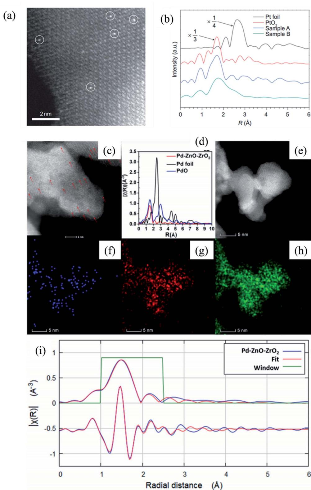
Fig. 14 (a) HAADF-STEM image and (b) EXAFS analysis of Pt<sub>1</sub>/FeO<sub>x</sub> catalyst; (c)–(i) HAADF-STEM, XANES, EXAFS and corresponding EDX mapping of Pd SAC. This figure has been adapted/reproduced from ref. 3 and 147 with permission from Nature Publishing Group and Springer Nature, copyright 2011 and 2020.
