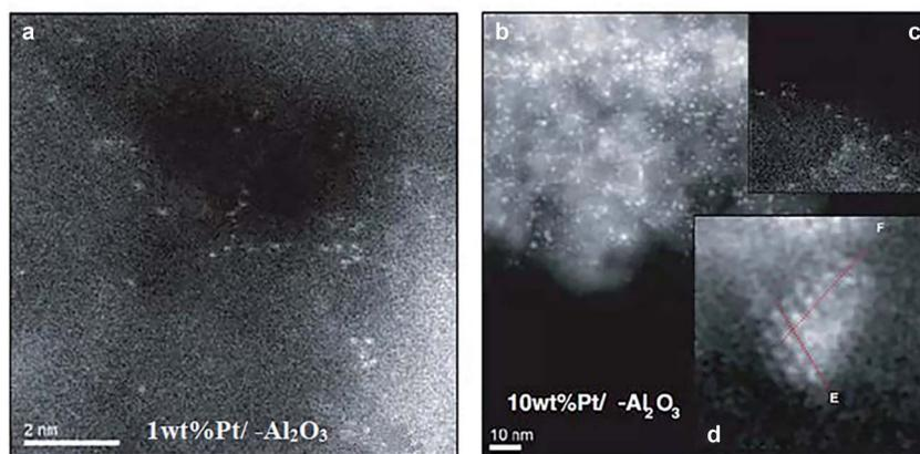
Fig. 9 HAADF-STEM images of (a) 1 wt% Pt/ $\gamma$ -Al<sub>2</sub>O<sub>3</sub> and (b) 10 wt% Pt/ $\gamma$ -Al<sub>2</sub>O<sub>3</sub>. The insets in Fig. 8b showed the presence of (c) atomically dispersed Pt and (d) Pt cluster/nanoparticles. This figure has been adapted/reproduced from ref. 107 with permission from American Association for the Advancement of Science, copyright 2009.
