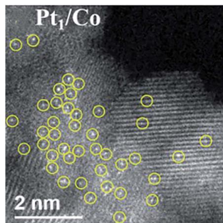
Fig. 7 HAADF-STEM image of Pt<sub>1</sub>/Co. This figure has been adapted/reproduced from ref. 94 with permission from American Chemical Society, copyright 2020.
