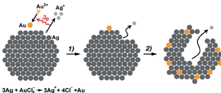
**Fig. 11** Schematic illustration of the galvanic replacement process (here the galvanic replacement of Ag by Au is shown as an example). This figure has been adapted/reproduced from ref. 126 with permission from Wiley-Blackwell, copyright 2013.
