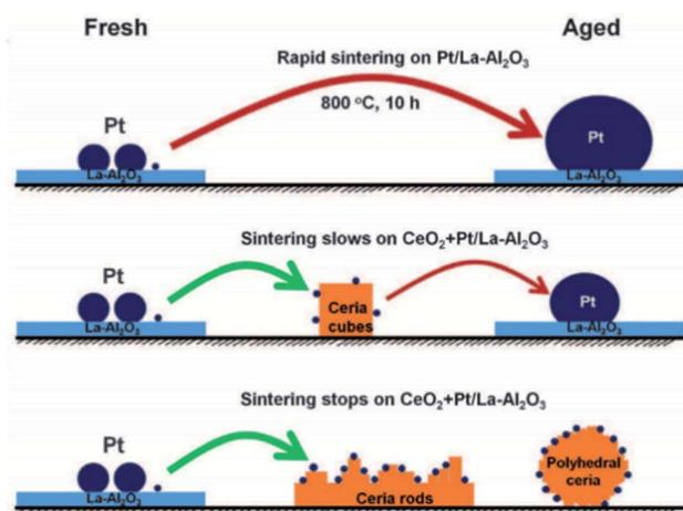
Fig. 4 Illustration of the synthesis of Pt<sub>1</sub>/CeO<sub>2</sub> SAC *via* the trapping of mobile Pt by CeO<sub>2</sub> due to the migration of Pt at high temperatures. This figure has been adapted/reproduced from ref. 87 with permission from American Association for the Advancement of Science, copyright 2016.
