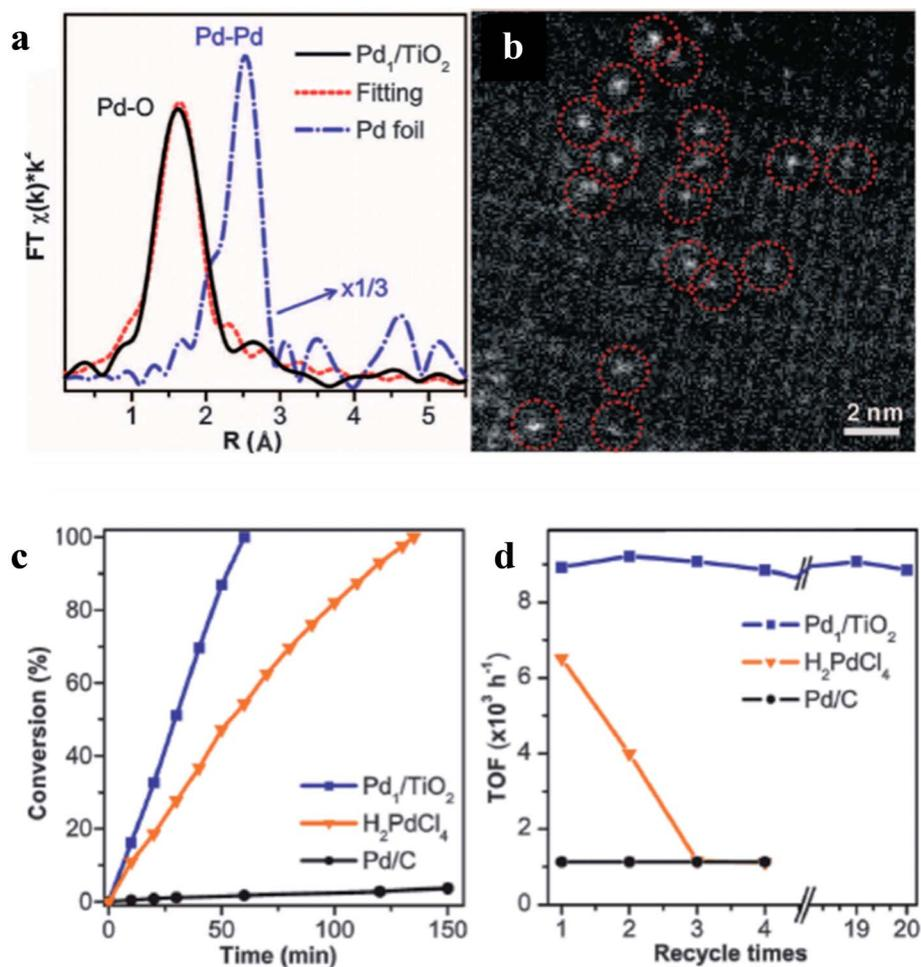
Fig. 10 (a) EXAFS analysis, (b) HAADF-STEM image as well as (c and d) catalytic performance of 1.5 wt%Pd/TiO<sub>2</sub> catalyst in styrene hydrogenation reaction. This figure has been adapted/reproduced from ref. 110 with permission from American Association for the Advancement of Science, copyright 2016.
