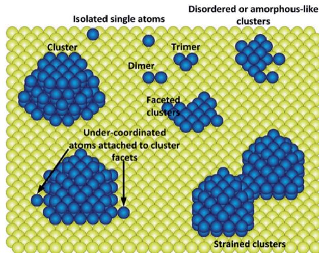
Fig. 16 Schematic illustration showing the co-existence of singly dispersed sites and continuously packed sites. This figure has been adapted/reproduced from ref. 32 with permission from American Chemical Society, copyright 2021.
