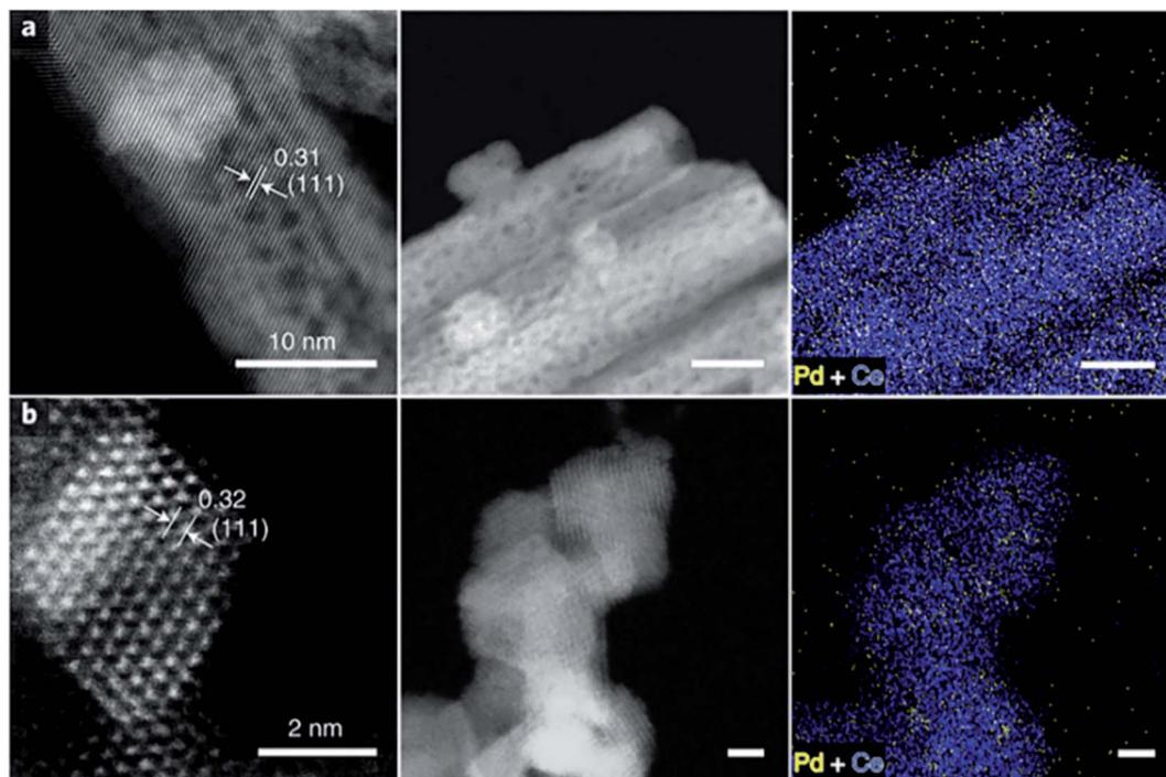
**Fig. 15** Structure HAADF-STEM image of Pd<sub>1</sub>/CeO<sub>2</sub> catalyst. (a) By impregnation method and (b) by flame spray pyrolysis. This figure has been adapted/reproduced from ref. 169 with permission from Nature Publishing Group, copyright 2021.
