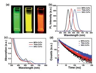
Fig. 1 Optical properties of aqueous solutions of MPA-CdTe QDs, TGA-CdTe QDs and NAC-CdTe QDs: (a) photographs taken under UV (365 nm) irradiation; (b) PL spectra measured under 400 nm excitation; (c) UV-Vis absorption spectra; (d) time-resolved PL decay curves.
