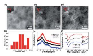
**Fig. 2** TEM and HRTEM (inset) images of (a) MPA-CdTe QDs, (b) TGA-CdTe QDs and (c) NAC-CdTe QDs. (d) Size distribution histogram of the MPA-CdTe QDs. (e) XRD patterns of CdTe QDs with different ligands. (f) FT-IR spectra of CdTe QDs with different ligands.
