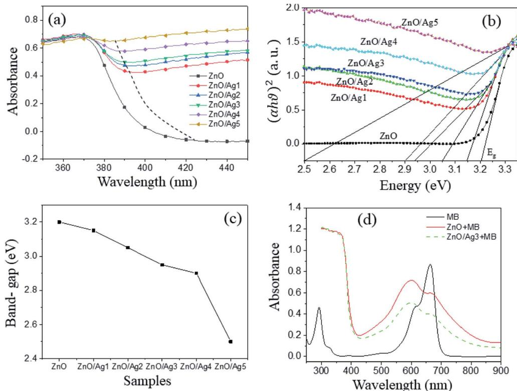
Fig. 5 (a) The UV-Vis absorption spectra of ZnO and ZnO/Ag<sub>x</sub> samples, (b) plot of  $(\alpha h\nu)^2$  versus  $h\nu$ , (c) the band-gap from 2.5 to 3.2 eV, (d) absorption spectra of MB alone (black line), of MB adsorbed on ZnO (red line) and ZnO/Ag<sub>3</sub> (dash line).
