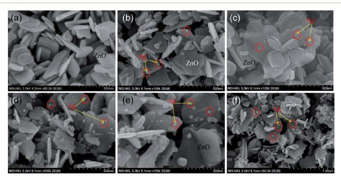
Fig. 1 SEM images of ZnO nanoplates (a) and ZnO/Ag1 (b), ZnO/Ag2 (c), ZnO/Ag3 (d), ZnO/Ag4 (e), and ZnO/Ag5 (f) grown with different amounts of  $AgNO_3$ .
