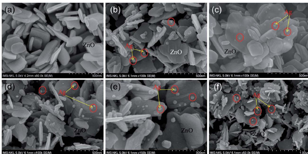
Fig. 1 SEM images of  $\text{ZnO}$  nanoplates (a) and  $\text{ZnO}/\text{Ag}_1$  (b),  $\text{ZnO}/\text{Ag}_2$  (c),  $\text{ZnO}/\text{Ag}_3$  (d),  $\text{ZnO}/\text{Ag}_4$  (e), and  $\text{ZnO}/\text{Ag}_5$  (f) grown with different amounts of  $\text{AgNO}_3$ .
