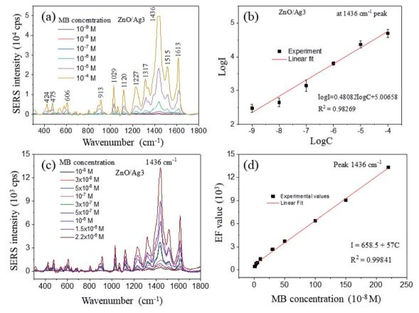
Fig. 8 (a) Raman spectra of MB adsorbed on ZnO/Ag3 at concentrations ranging from  $10^{-9}$  M to  $10^{-4}$  M, (b) the linear relationship between the log / and log C of the 1436 cm $^{-1}$  peak, where / is the SERS intensity and C is the MB concentration, (c) Raman spectra of MB adsorbed on ZnO/Ag3 with different concentrations from  $10^{-8}$  M to  $2.2 \times 10^{-6}$  M, (d) the linear relationship between SERS intensity and MB concentration.
