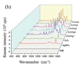
Fig. 7 Raman spectra of MB on Si substrate (a), MB adsorbed on AgNPs, ZnO NPls, ZnO/Ag (b), MB concentration in all experiments as 10<sup>-4</sup> M.
