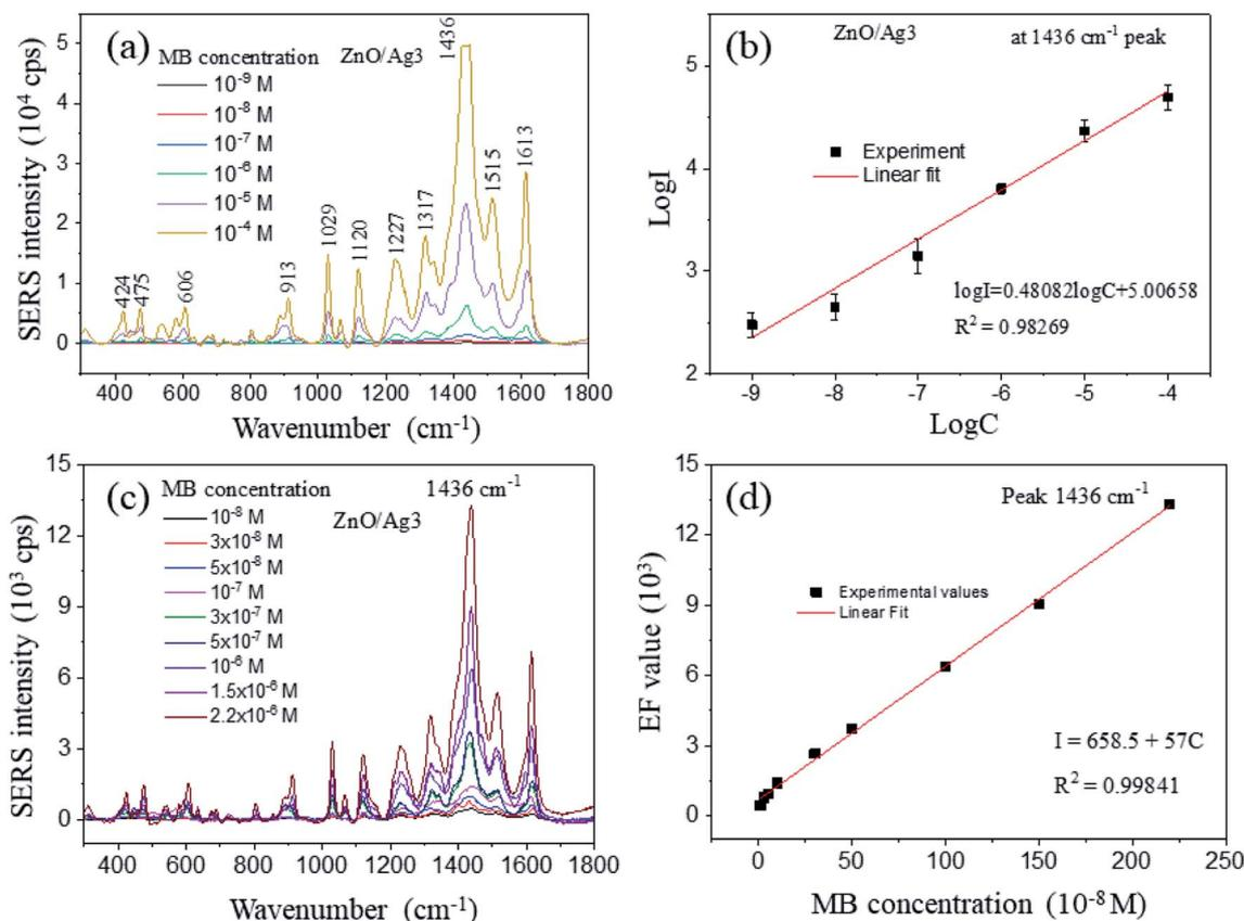
Fig. 8 (a) Raman spectra of MB adsorbed on ZnO/Ag3 at concentrations ranging from  $10^{-9}$  M to  $10^{-4}$  M, (b) the linear relationship between the  $\log I$  and  $\log C$  of the  $1436 \text{ cm}^{-1}$  peak, where  $I$  is the SERS intensity and  $C$  is the MB concentration, (c) Raman spectra of MB adsorbed on ZnO/Ag3 with different concentrations from  $10^{-8}$  M to  $2.2 \times 10^{-6}$  M, (d) the linear relationship between SERS intensity and MB concentration.
