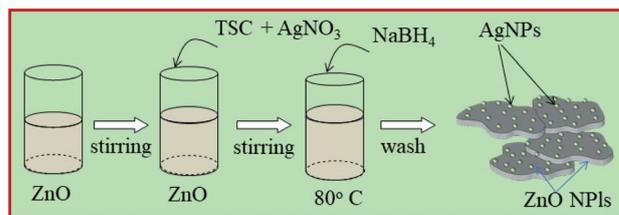
Scheme 1 Schematic illustration of ZnO/Ag hybrid preparation process.
