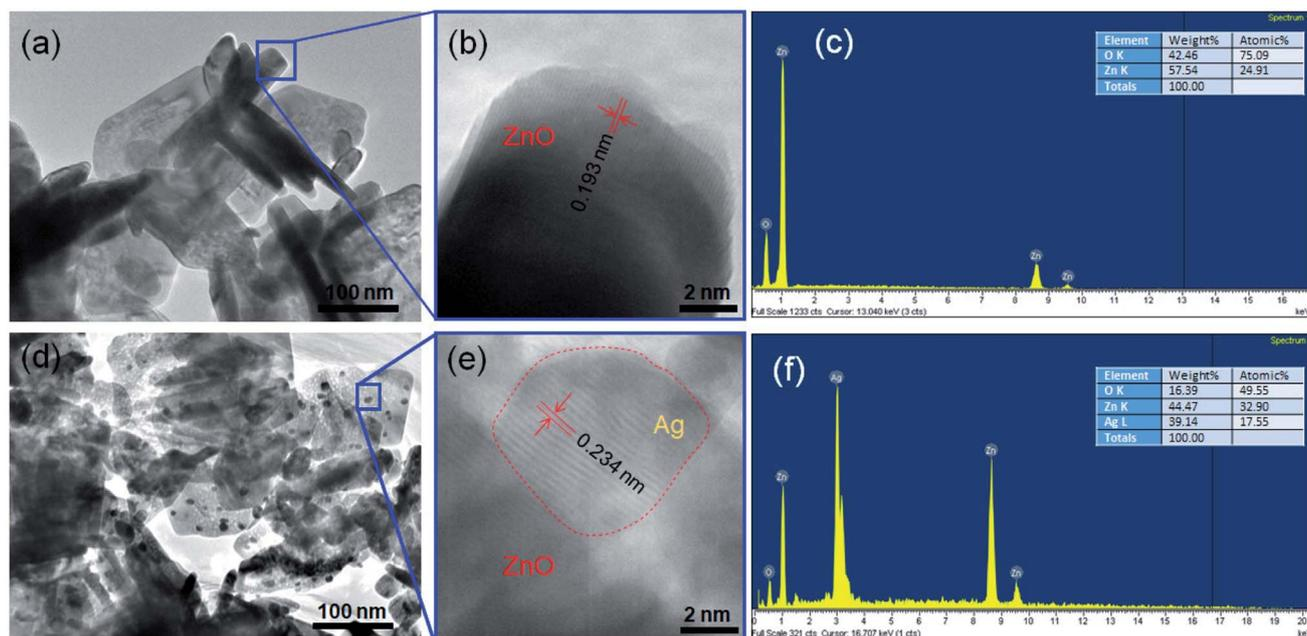
Fig. 4 (a) Typical TEM and (b) HRTEM images of ZnO, (d) TEM and (e) HRTEM images of ZnO/Ag<sub>3</sub> and corresponding spot-profile EDS spectra of (c) pure ZnO, (f) ZnO/Ag<sub>3</sub>.
