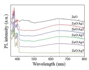
Fig. 6 Photoluminescence (PL) spectra of ZnO and ZnO/Ag excited at 345 nm.
