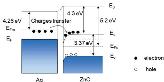
Scheme 2 Energy band diagram of ZnO/Ag interface showing the electron transfer between Ag and ZnO.<sup>61</sup>
