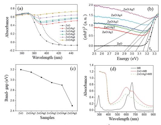
Fig. 5 (a) The UV-Vis absorption spectra of ZnO and ZnO/Agx samples, (b) plot of  $(\alpha h v)^2$  versus hv, (c) the band-gap from 2.5 to 3.2 eV, (d) absorption spectra of MB alone (black line), of MB adsorbed on ZnO (red line) and ZnO/Ag3 (dash line).
