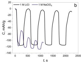
Fig. 2 (a) CV curves of the synthesized material in 1 M LiCl and 1 M NaClO<sub>4</sub> electrolytes at 5 mV s<sup>-1</sup>; (b) time capacity dependence curves obtained by CV curve integration.
