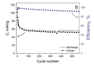
Fig. 4 Cycling stability tests of the synthesized material performed by (a) CV mode at 5 mV s $^{-1}$  and (b) GC mode at 1 A g $^{-1}$ .
