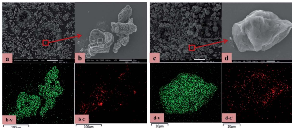
Fig. 6 SEM-EDS: (a) the precursor obtained by microwave-assisted; (b) the partially enlarged view of the edge of the precursor obtained by microwave-assisted; (c) the precursor obtained by vanadium precipitation with adding C; (d) the partially enlarged view of the edge of the precursor obtained by vanadium precipitation with adding C.
