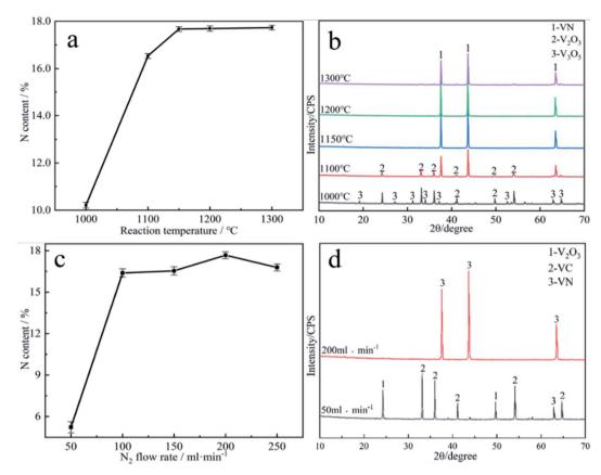
Fig. 4 Effect of reduction nitride conditions on the N content of vanadium nitride: (a) reaction temperature; (b) the physical phases of the products at each reaction temperature condition; (c)  $N_2$  flow rate; (d) the physical phases of the products at different  $N_2$  flow rate.
