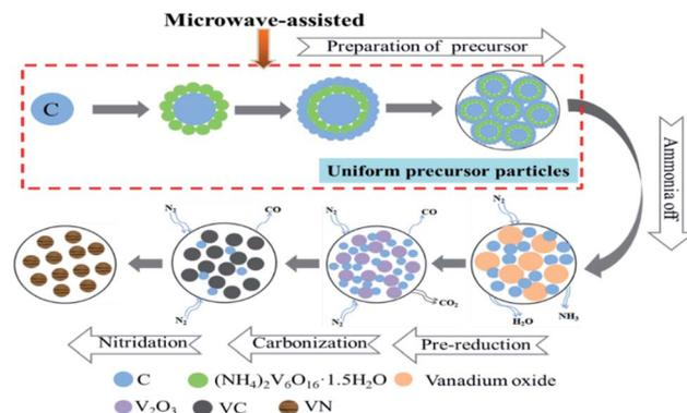
Fig. 9 Mechanism of preparation of vanadium nitride.
