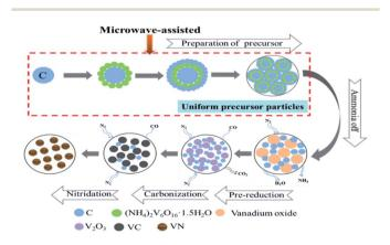
Fig. 9 Mechanism of preparation of vanadium nitride.
