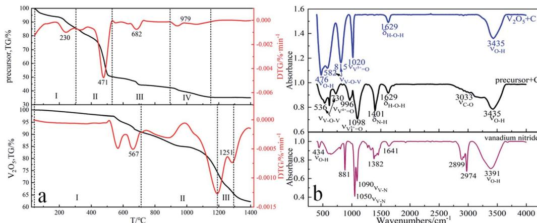
Fig. 8 (a) TG-DTG curves of precursor and  $V_2O_5$  from 20 °C to 1400 °C under  $N_2$  atmosphere; (b) FTIR analysis of precursor,  $V_2O_5$  and vanadium nitride.
