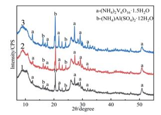
Fig. 5 XRD patterns of the precursor: (1) the product precipitated directly from vanadium solution; (2) the precursor obtained by vanadium precipitation with adding C; (3) the precursor obtained by microwave-assisted.
