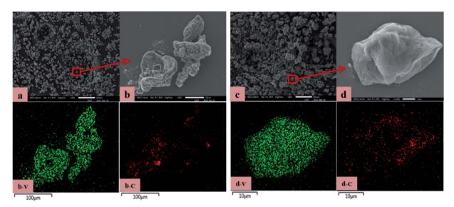
Fig. 6 SEM-EDS: (a) he precursor obtained by microwave-assisted; (b) the partially enlarged view of the edge of the precursor obtained by microwave-assisted; (c) the precursor obtained by vanadium precipitation with adding C; (d) the partially enlarged view of the edge of the precursor obtained by vanadium precipitation with adding C.
