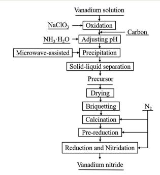
Fig. 1 Process flow sheet for preparation of vanadium nitride.
