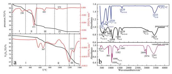
Fig. 8 (a) TG-DTG curves of precursor and  $V_2O_5$  from 20 °C to 1400 °C under  $N_2$  atmosphere; (b) FTIR analysis of precursor,  $V_2O_5$  and vanadium
