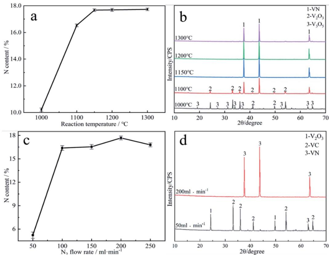
Fig. 4 Effect of reduction nitride conditions on the N content of vanadium nitride: (a) reaction temperature; (b) the physical phases of the products at each reaction temperature condition; (c) N<sub>2</sub> flow rate; (d) the physical phases of the products at different N<sub>2</sub> flow rate.
