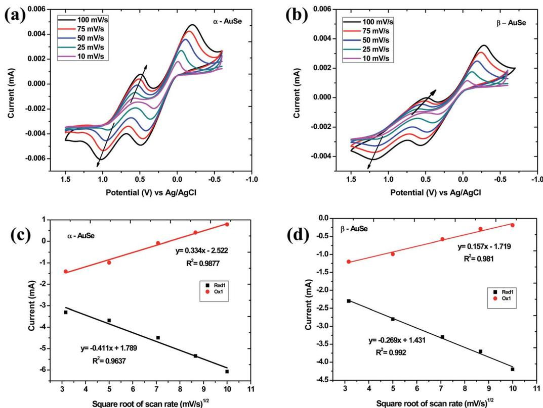
Fig. 6 Cyclic voltammograms for (a)  $\alpha$ -AuSe and (b)  $\beta$ -AuSe CEs at varying scan rates from  $10 \text{ mV s}^{-1}$  to  $100 \text{ mV s}^{-1}$ . Dependence of anodic and cathodic peak currents on square root of scan rates for (c)  $\alpha$ -AuSe and (d)  $\beta$ -AuSe CEs.
