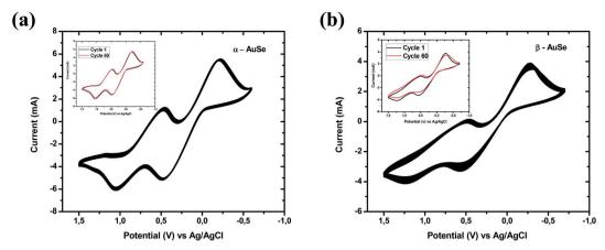
Fig. 7 Cyclic voltammograms for, (a)  $\alpha$ -AuSe and (b)  $\beta$ -AuSe CEs for 60 consecutive cycles, with inserts showing the 1<sup>st</sup> and the 60<sup>th</sup> cycle for both electrodes.
