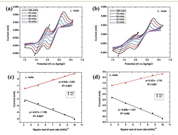
Fig. 6 Cyclic voltammograms for (a)  $\alpha$ -AuSe and (b)  $\beta$ -AuSe CEs at varying scan rates from 10 mV s<sup>-1</sup> to 100 mV s<sup>-1</sup>. Dependence of anodic and cathodic peak currents on square root of scan rates for (c)  $\alpha$ -AuSe and (d)  $\beta$ -AuSe CEs.
