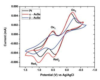
Fig. 5 Cyclic voltammograms of the Pt,  $\alpha$ -AuSe and  $\beta$ -AuSe counter electrodes at a scan rate of 100 mV s<sup>-1</sup> for the I<sup>-</sup>/I<sub>3</sub><sup>-</sup> redox couple.
