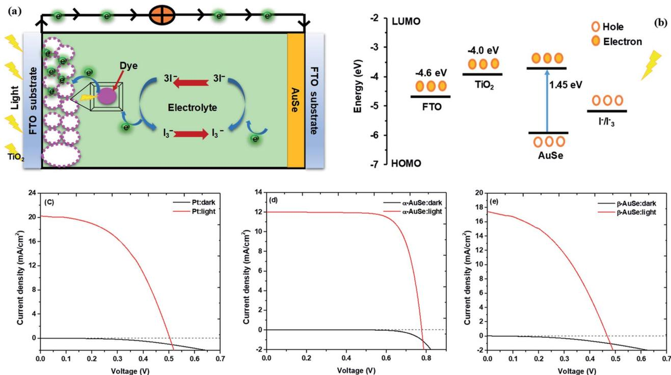
Fig. 9 (a) Schematic of a DSSC, (b) energy diagram of the DSSC, (c)  $J$ - $V$  curves of DSSCs with Pt, (d)  $\alpha$ -AuSe and (e)  $\beta$ -AuSe CEs in the dark and under 100  $\text{mW cm}^{-2}$  illumination.
