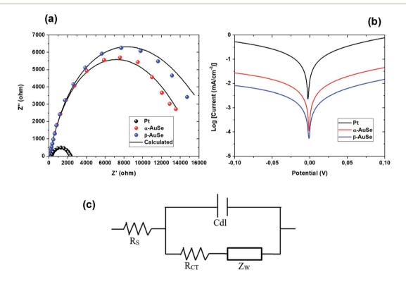
Fig. 8 (a) Nyquist plots, (b) Tafel polarization curves for the symmetric cells fabricated with Pt,  $\alpha$ -AuSe and  $\beta$ -AuSe CEs and (c) the equivalent circuit.
