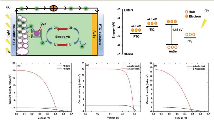
Fig. 9 (a) Schematic of a DSSC, (b) energy diagram of the DSCC, (c) J-V curves of DSSCs with Pt, (d)  $\alpha$ -AuSe and (e)  $\beta$ -AuSe CEs in the dark and under 100 mW cm<sup>-2</sup> illumination.
