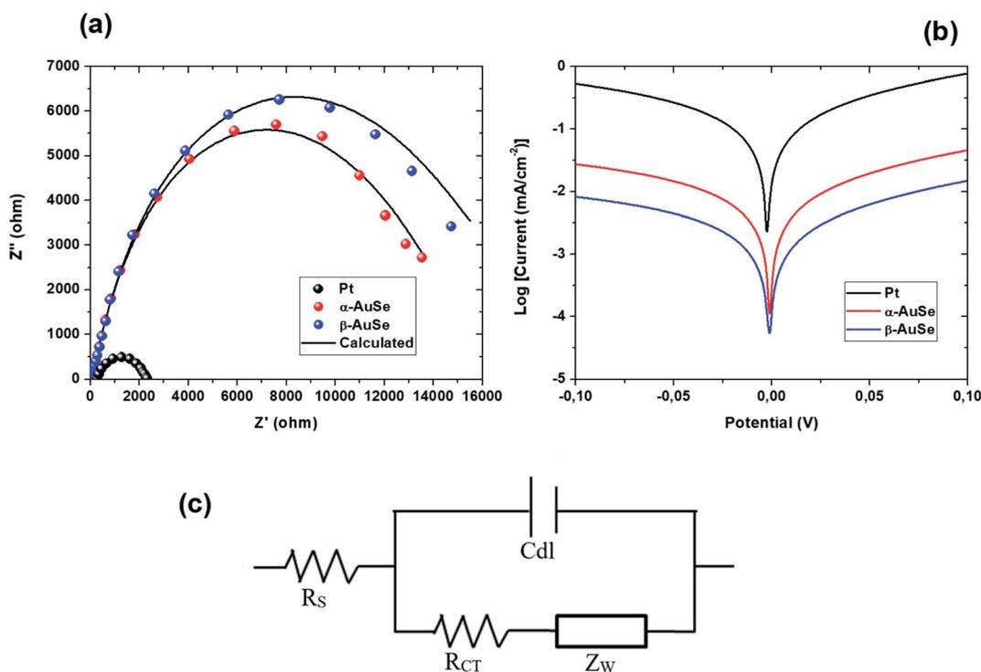
Fig. 8 (a) Nyquist plots, (b) Tafel polarization curves for the symmetric cells fabricated with Pt,  $\alpha$ -AuSe and  $\beta$ -AuSe CE and (c) the equivalent circuit.
