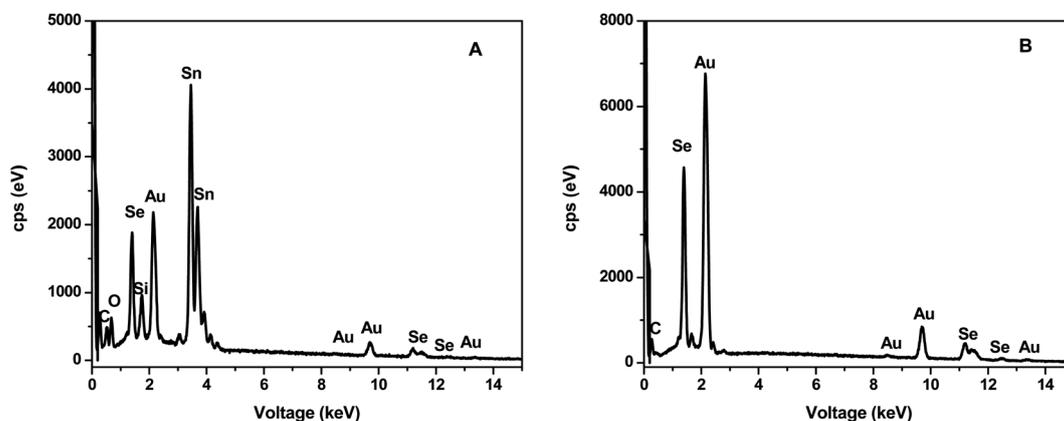
Fig. 4 SEM-EDS of (A)  $\alpha$ -AuSe-CE and (B)  $\beta$ -AuSe-CE showing the elemental composition of the materials on the FTO glass substrates.
