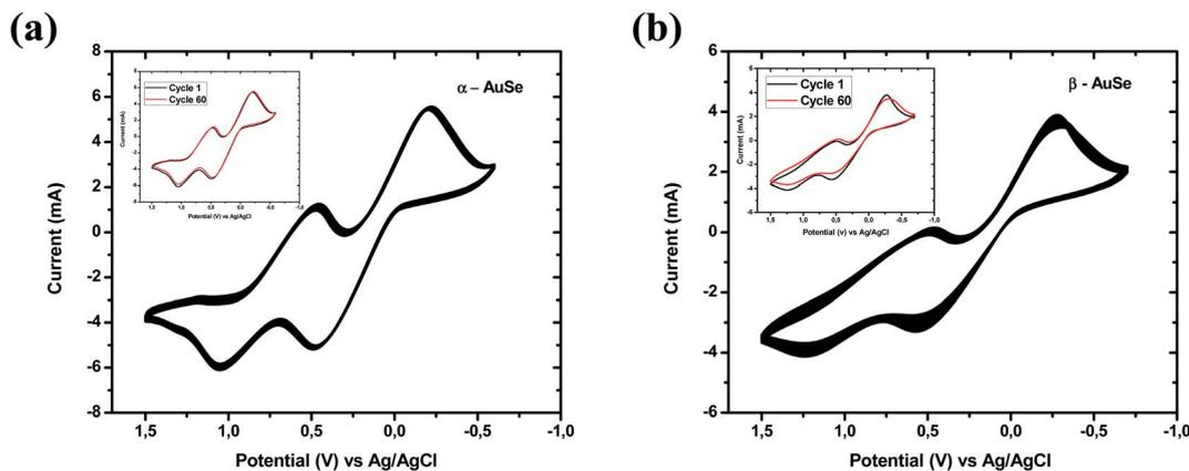
Fig. 7 Cyclic voltammograms for, (a)  $\alpha$ -AuSe and (b)  $\beta$ -AuSe CE for 60 consecutive cycles, with inserts showing the 1<sup>st</sup> and the 60<sup>th</sup> cycle for both electrodes.
