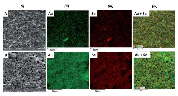
(i) SEM images of (A) α-AuSe and (B) β-AuSe counter electrodes. Elemental mapping of (ii) Au, (iii) Se and (iv) summed mapping of Au and
