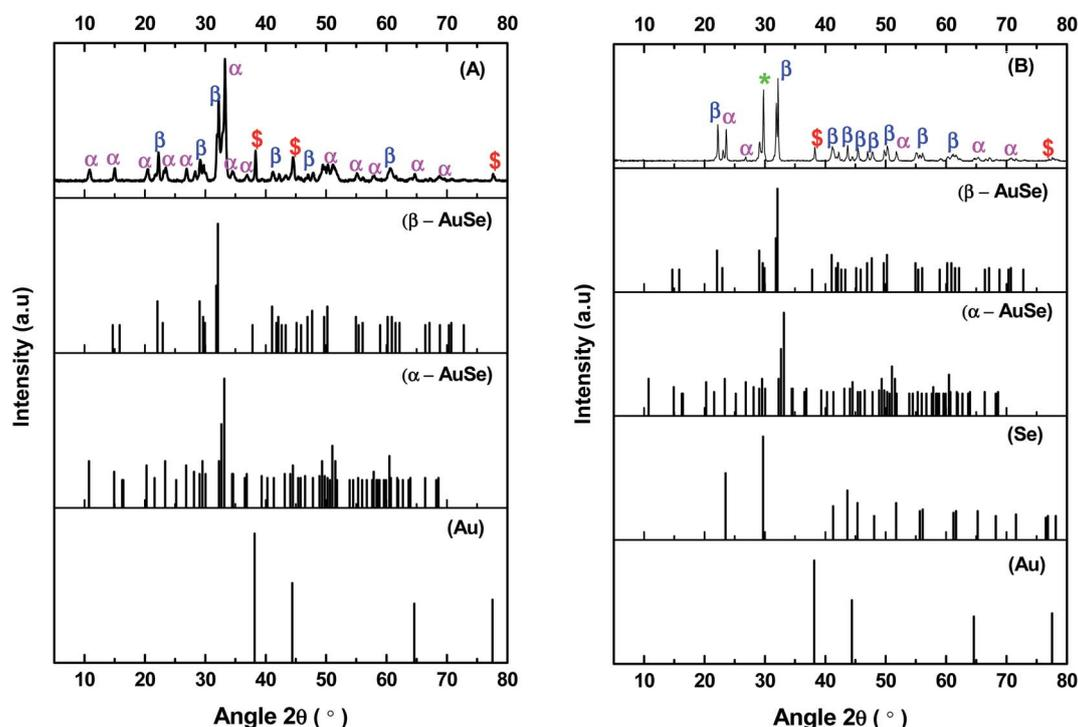
Fig. 1 Powder X-ray diffraction patterns of as-synthesized AuSe matched to standard powder patterns of  $\alpha$ -AuSe (A),  $\beta$ -AuSe (B), and elemental Au & elemental Se (key:  $\alpha$  =  $\alpha$ -AuSe,  $\beta$  =  $\beta$ -AuSe, \$ = elemental Au and \* = elemental Se).
