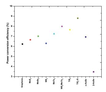
Fig. 10 A comparison plot showing the trend in power conversion efficiencies (PCEs) of a few 2-dimensional layered transition metal chalcogenides.
