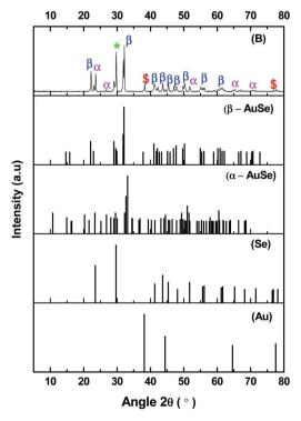
Fig. 1 Powder X-ray diffraction patterns of as-synthesized AuSe matched to standard powder patterns of  $\alpha$ -AuSe (A),  $\beta$ -AuSe (B), and elemental Au  $\delta$  elemental Se (key:  $\alpha = \alpha$ -AuSe,  $\beta = \beta$ -AuSe,  $\xi$  = elemental Au and \* = elemental Se).
