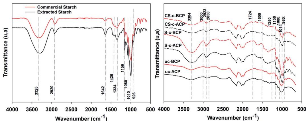
Fig. 4 FTIR spectra of the starches and elaborated cellulosic papers.
