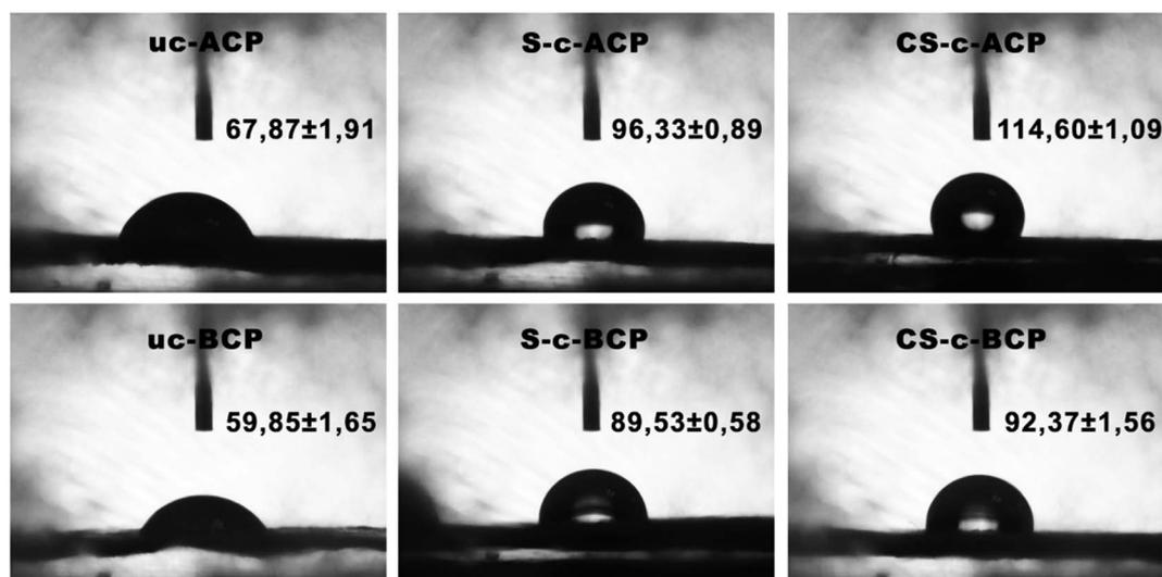
Fig. 7 Contact angle of the elaborated cellulosic papers.
