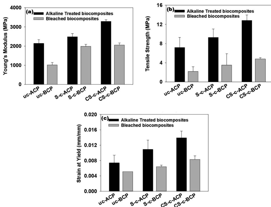
Fig. 9 Tensile properties of the elaborated cellulosic papers.
