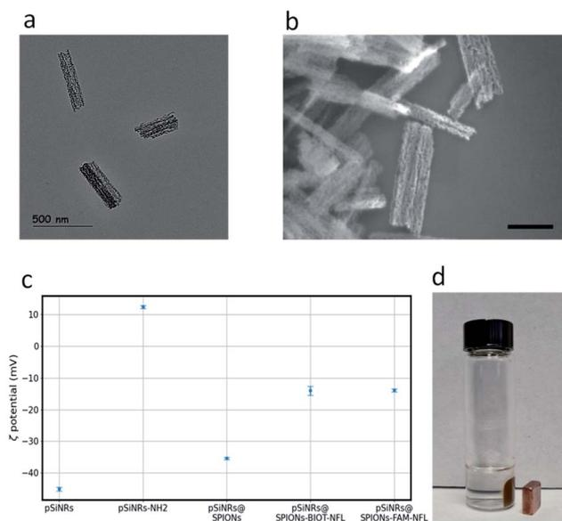
Fig. 2 (a) Transmission electron microscopy image of pSiNRs. Scale bar: 500 nm (b) scanning electron microscopy image of pSiNRs. Scale bar: 200 nm (c)  $\zeta$ -potential measurements at each step of modifications. Bars represent mean  $\pm$  SD ( $n = 3$ ). (d) Photograph of magnetic pSiNRs under magnetic field.
