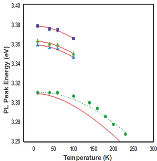
Fig. 14 The temperature dependence of the peak energies for the  $\text{FX}_A$  emission (solid squares), the  $\text{D}^\circ\text{X}$  emission (solid triangles), BF emission (reverse solid triangles) and the BF-1LO emission (solid circles). Solid lines are calculated using Varshni's formula. The dotted line is calculated using the formula  $h\nu = E_g - E_D + k_B T$ .
