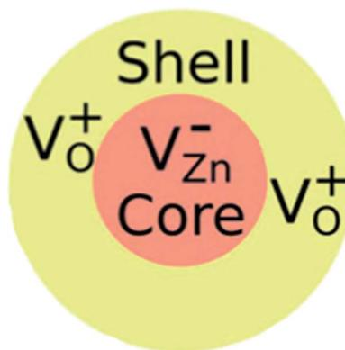
Fig. 11 The surface/shell defects is attributed to an unpaired electron-trapped oxygen vacancy ( $\text{V}_\text{O}$ ) site and the core defects is attributed to  $\text{V}_{\text{Zn}}^-$  centers [Shankari Nadupalli].
