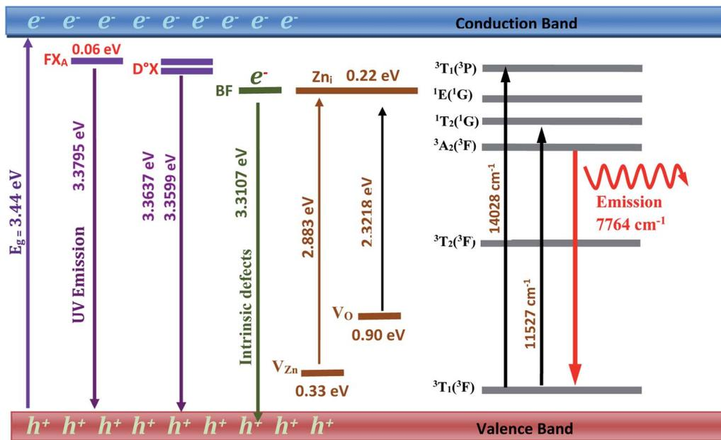
Fig. 15 UV-Vis-near infrared energy level diagram of ZnO:Ni<sup>2+</sup> NPs.
