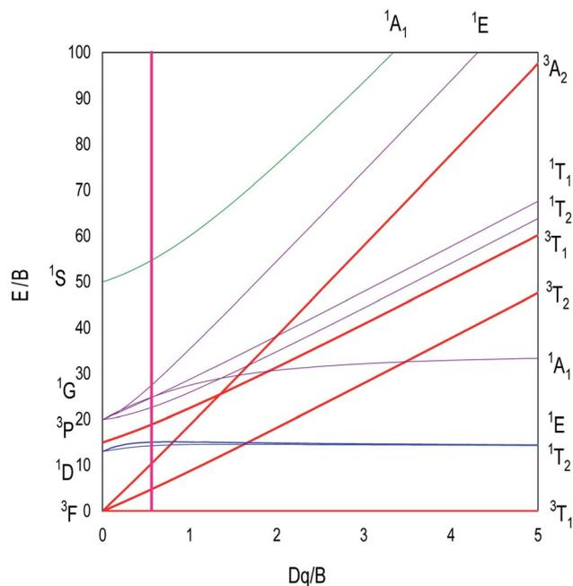
Fig. 12 Tanabe–Sugano diagram for tetrahedral coordinated  $\text{Ni}^{2+}$  ion with  $C/B = 4.64$ . The vertical line with  $Dq/B = 0.57$  represents the case of  $\text{ZnO}:\text{Ni}^{2+}$  NPs.
