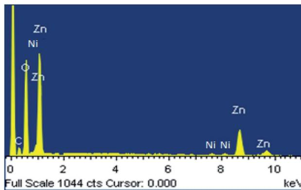
Fig. 2 EDX spectrum of Ni doped ZnO NPs.
