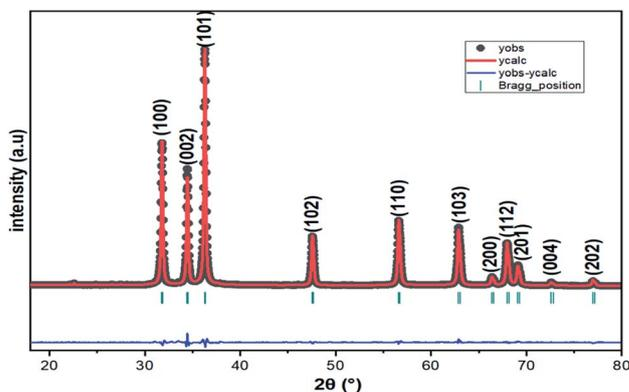
Fig. 3 Powder X-ray diffraction pattern of  $Zn_{0.95}Ni_{0.05}O$  NPs.
