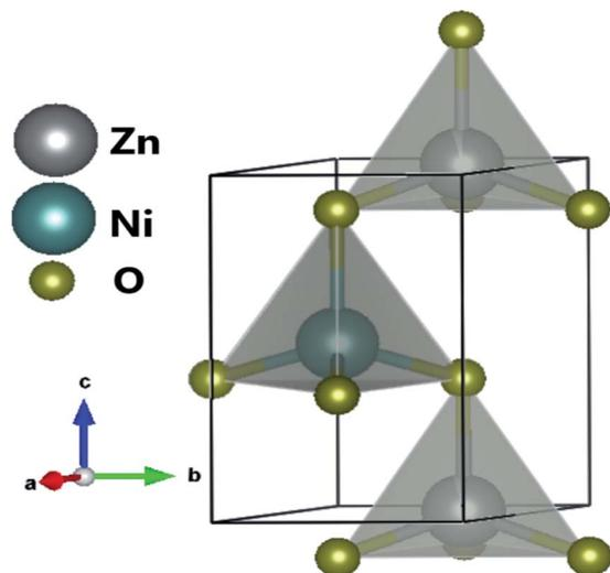
Fig. 4 Crystal structure of ZnO doped with Ni<sup>2+</sup>.
