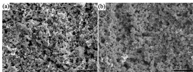
Fig. 8 SEM images of the Sr-npSi anode (a) before and (b) after 100 charge/discharge cycles at a current density of  $50 \text{ mA g}^{-1}$  for the initial two cycles and at  $0.5 \text{ A g}^{-1}$  in the following cycles.
