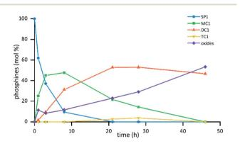
Fig. 1 Evolution of the reaction of hydrolysis in phosphine SP1 in sulfuric acid with time. Reaction conditions [SP1]: = 0.15 M, [H<sub>3</sub>BO<sub>3</sub>] = 0.8 M, [SO<sub>3</sub>] = 10.5 M.
