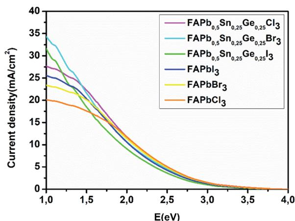
Fig. 5 Short-circuit current density of FAPbX<sub>3</sub> and FAPb<sub>0.5</sub>Sn<sub>0.25</sub>Ge<sub>0.25</sub>X<sub>3</sub>.
