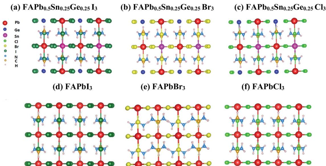
Fig. 1 Optimized tetragonal structures of  $\text{FAPb}_{0.5}\text{Sn}_{0.25}\text{Ge}_{0.25}\text{X}_3$  and  $\text{FAPbX}_3$ .
