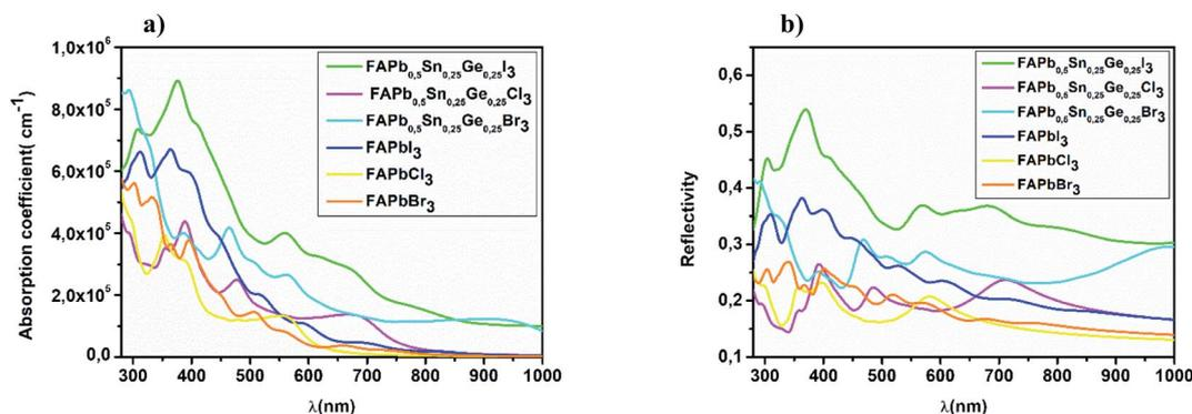
Fig. 4 Spectral (a) absorption coefficient and (b) reflectivity of FAPb<sub>0.5</sub>Sn<sub>0.25</sub>Ge<sub>0.25</sub>X<sub>3</sub>.
