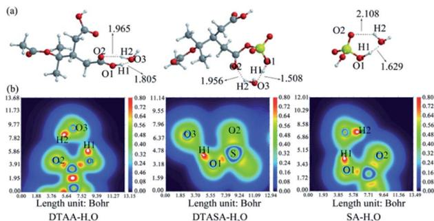
Fig. 3 (a) The most stable configurations at M06-2X/6-311+G(3df,3pd) level of theory and (b) corresponding color-filled LOL map of clusters DTAA-H<sub>2</sub>O, DTASA-H<sub>2</sub>O and SA-H<sub>2</sub>O. Dashed lines represent the hydrogen bonds, and all distances are in angstroms. The H, C, O and S atoms are represented as white, gray, red and yellow spheres, respectively.
