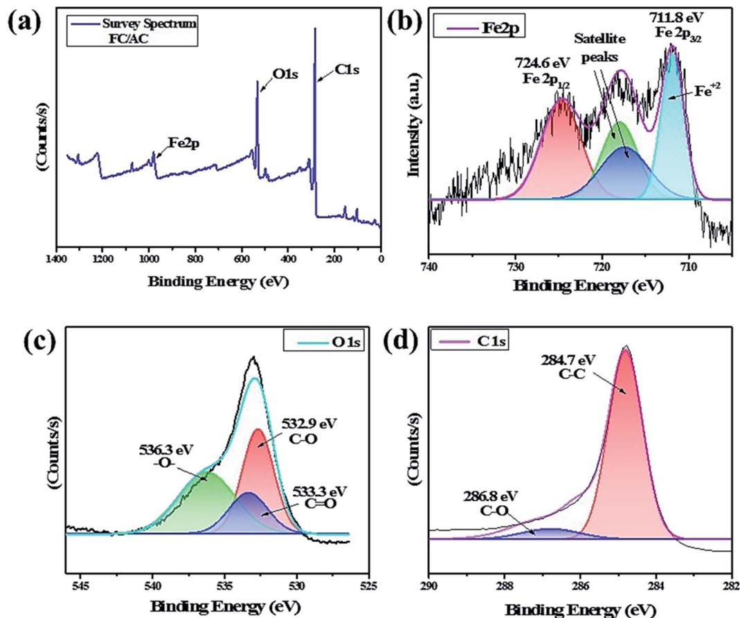
Fig. 6 (a) Survey spectrum of FC/AC, deconvoluted spectra of (b) Fe2p, (c) O1s and (d) C1s.
