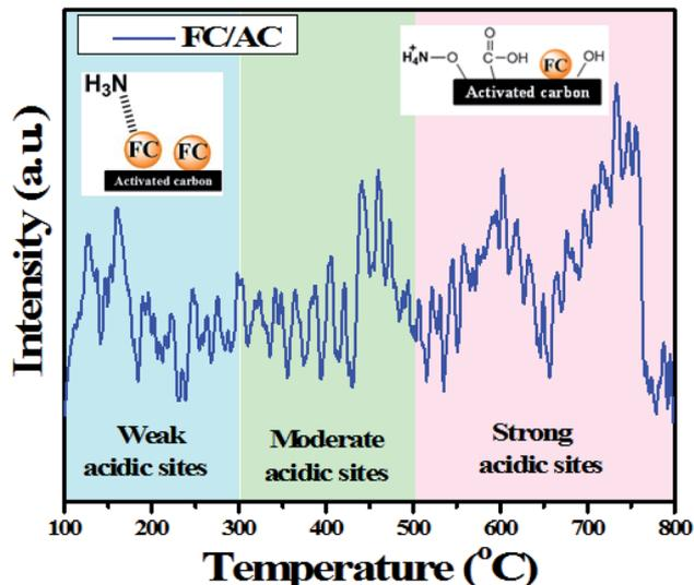
Fig. 8 NH<sub>3</sub>-TPD analysis of FC/AC catalyst.
