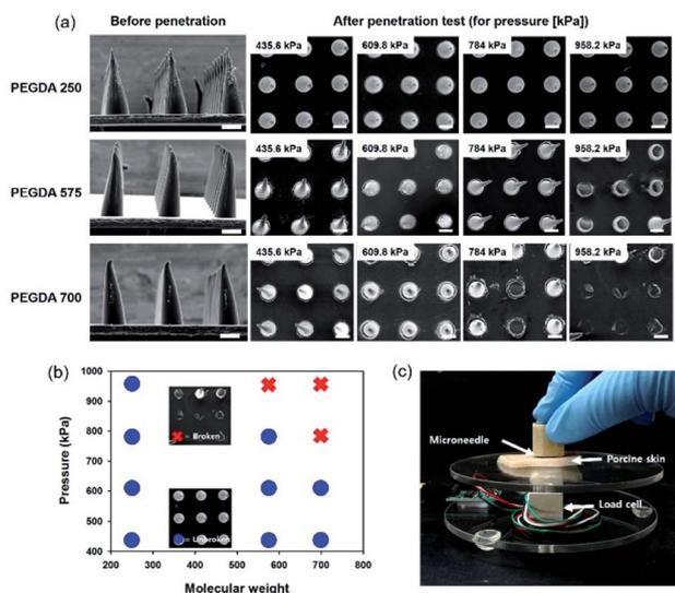
**Fig. 5** (a) SEM images of MNs before and after the penetration test on the porcine skin according to the PEGDA molecular weight and shear pressure. (b) A graph showing the condition to be stable or broken after the penetration test according to the PEGDA molecular weight and shear pressure. (c) An experimental setup to measure the applied force to MNs using a load cell. Scale bars represent 100  $\mu\text{m}$ .
