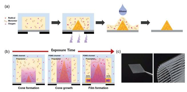
Fig. 1 (a) Schematic illustration of the fabrication process of cone-shaped MNs using FRP. (b) Schematic illustration of formation of different MN shape asshapes with increasing exposure time increases. (c) Photographs of fabricated cone-shaped MNs, bonded on a flexible PET substrate.
