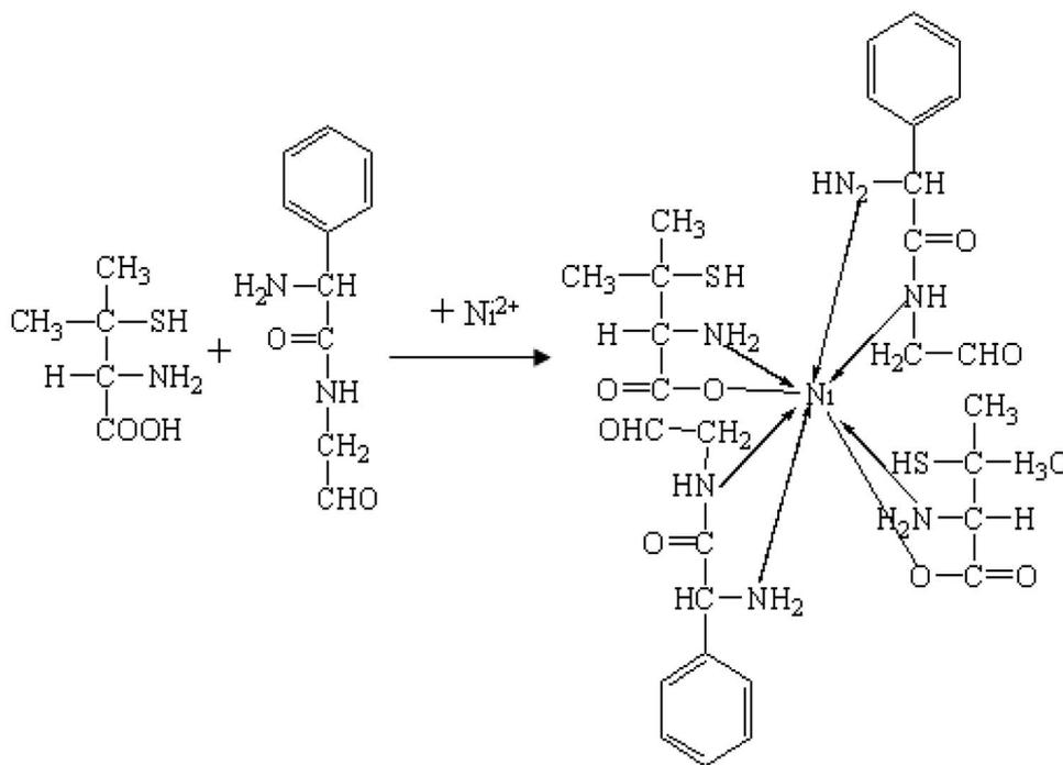
Fig. 9 Reaction mechanism of the complex formation.
