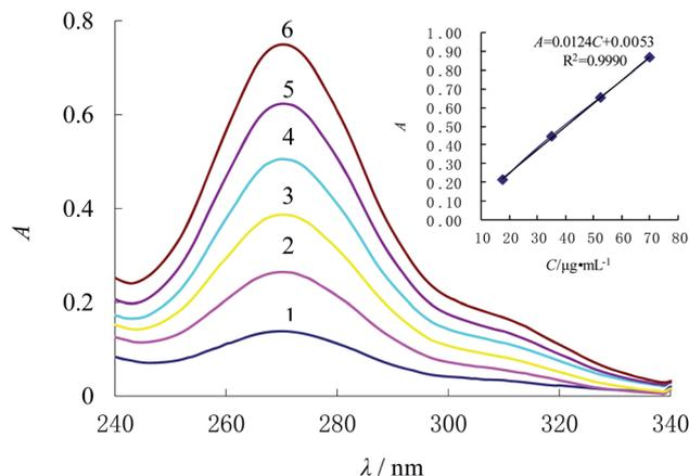
**Fig. 3** Absorption spectra of the complex for different concentrations of ampicillin with 0.20 mL 1% ammonium hydroxide and  $2.00 \times 10^{-4}$  mol L $^{-1}$  Ni $^{2+}$ . From 1 to 6, ampicillin is  $6.00 \times 10^{-5}$  mol L $^{-1}$ ,  $1.20 \times 10^{-4}$  mol L $^{-1}$ ,  $1.80 \times 10^{-4}$  mol L $^{-1}$ ,  $2.40 \times 10^{-4}$  mol L $^{-1}$ ,  $3.00 \times 10^{-4}$  mol L $^{-1}$ ,  $3.60 \times 10^{-4}$  mol L $^{-1}$ , respectively.
